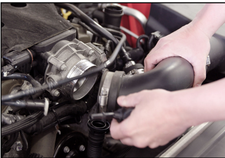
10. Remove the INLET/DUCT from the throttle body.
