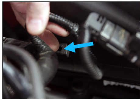
11. Remove wire clip from air induction housing.
