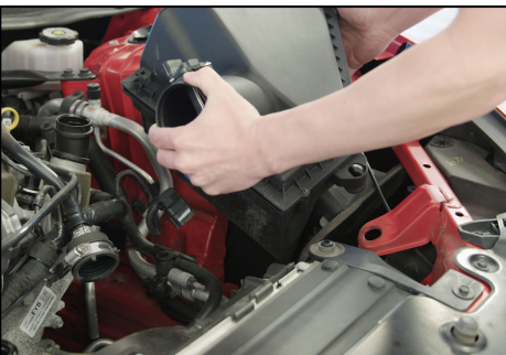
13. Gently remove the production air induction housing.
