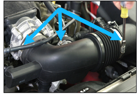
6. Loosen hose clamps with 8 mm nut driver.
