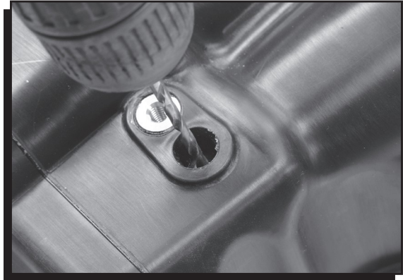
Figure 6 Drilling the MAP Sensor Hole.
