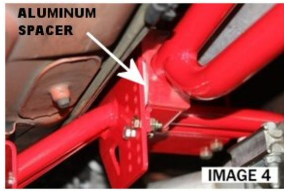
10. Choose a desired mounting hole then connect the saddle to the BMR cross-member, “sandwiching” the supplied aluminum shim between the bushing and the cross-member mount as shown in **IMAGE 4**. The high-clearance square shoulder bolts go in the top slotted holes of the cross-member and the 5/16” hex bolts go in the bottom (2) holes of the cross-member. Use the smaller 5/16” washers under the nuts.
