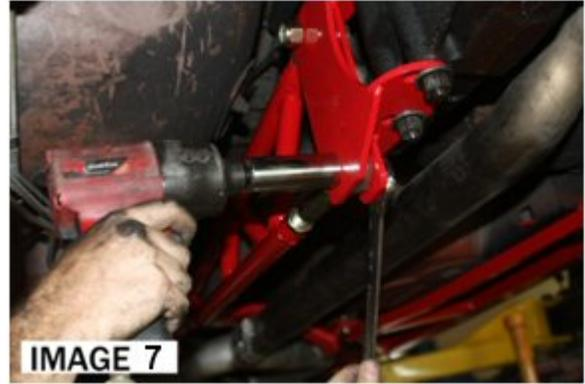
5. We recommend 1-2 degrees down (pinion pointing downwards) for automatic-equipped cars and 2-3 degrees down for manual-equipped cars. To adjust your pinion angle, simply turn the rear adjuster on the torque arm until you get your desired settings.
