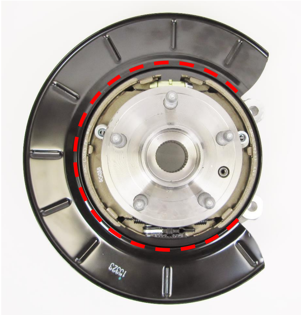
Figure 1: Trim the debris shield along the dashed line.
