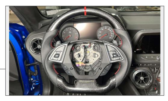
Align the steering wheel to the vehicle, and route the clockspring harness through the steering wheel. Fit the steering wheel to the steering column and secure into place using the original T-50 Torx bolt.
