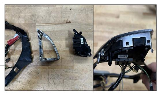
Unplug the wiring harness from the cruise control switches.
