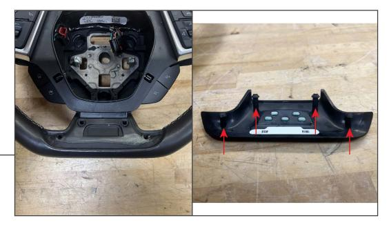
Begin to disassemble the steering wheel by removing the lower trim panel using a plastic trim tool around the perimeter of the trim.
