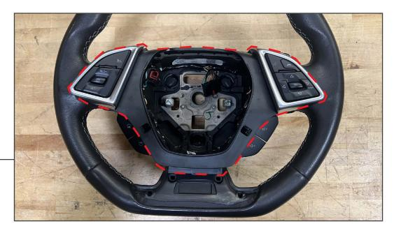
Using a plastic pry tool, gently pry around the perimeter of the steering wheel center section. This assembly is secured using large plastic dowels in the foam. These dowels can be difficult to remove and sometimes require additional pressure/force to dislodge.
