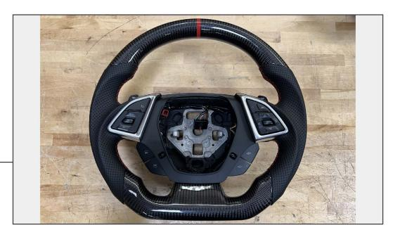
Align the center section to the new steering wheel, and plug in the rear paddle switches. Press the center section into the steering wheel. During installation, ensure the wiring harnesses/connectors are properly routed, and connectors are properly secured into place.
