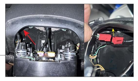
With the air bag pulled away from the steering wheel, locate the red connector along the LH top edge of the air bag area. Using a small flathead screwdriver, lift the steering wheel side red connector tab while pulling the air bag connector away from the steering wheel connector.
