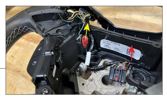
If necessary, push the foam securing the red connector in place, and lift the red connector from the foam.
