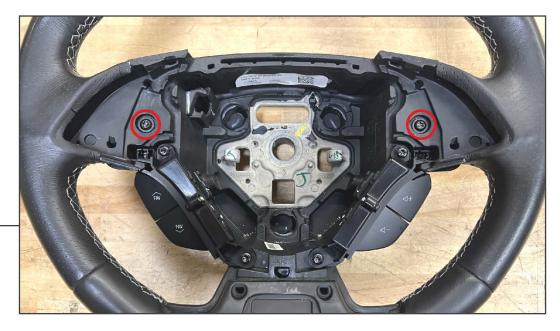
Remove (2) T-25 Torx bolts from the rear paddles. Lift the paddles from the rear of the steering wheel and set aside with the hardware.
