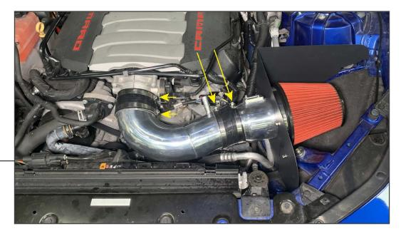
Install (1) coupler and (2) clamps to the MAF housing. Then, install (1) coupler and (2) clamps to the intake tube. Then, fit the intake tube to the MAF housing and throttle body. Ensure both couplers are properly fitted, and tighten the clamps to secure the intake tube into place.
