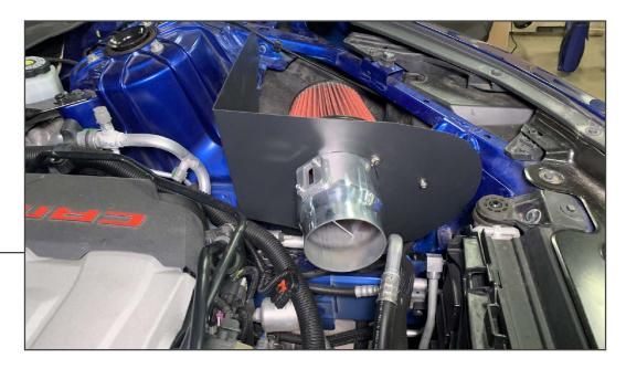
Secure the MAF housing to the intake heat shield using (2) M6 x 20mm Hex bolts, (2) M6 lock washers, and (2) M6 flat washers into the MAF housing threaded inserts.
