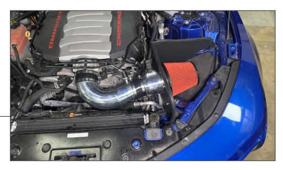
Plug in the MAF sensor harness into the MAF sensor. Route the harness away from any hot/moving components. Ensure all clamps are secure. Route the included weatherstripping around the perimeter of the heat shield, trim to fit as necessary.
