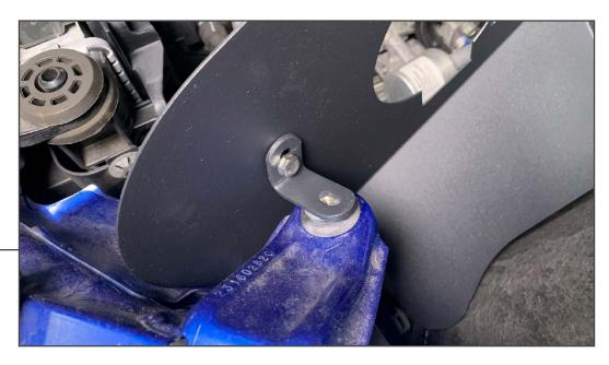
Secure the included heat shield mounting bracket to the heat shield using (1) M6 x 15mm flange bolt, (1) M6 lock washer, (2) M6 flat washers, and (1) M6 nut. Then, secure the mounting bracket to the previously placed threaded insert using (1) M6 flange bolt, (1) M6 lock washer, and (1) M6 flat washer.
