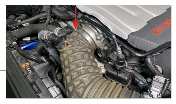
Loosen (1) 8mm clamp securing the intake tube to the throttle body.
