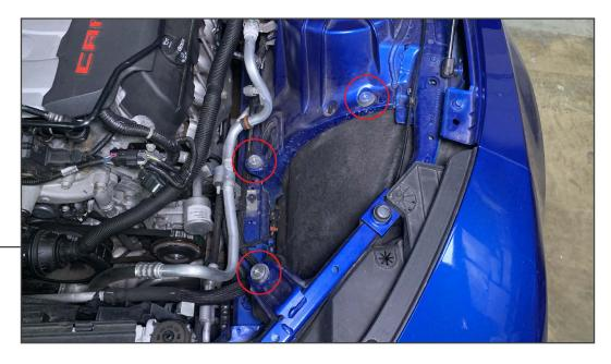
Fit the (3) M6 threaded inserts into the original air box rubber grommets.
