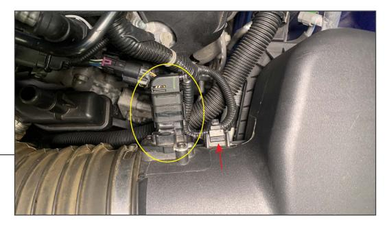
Unplug the vehicle MAF sensor, and unclip the wiring harness from the vehicle air box.
