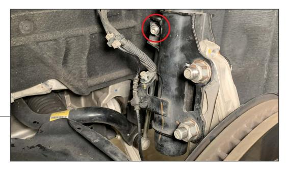
Remove the (1) 18mm nut from the top of the sway bar link attaching the sway bar to the vehicle strut.
