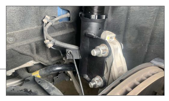
Lower the coilover lower mount moderately, then lift and align the vehicle steering knuckle to the coilover assembly. Secure the steering knuckle and brake line using the original hardware. Secure the ABS line into the mounting bracket on the coilover.
