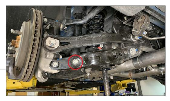
Place a floor jack under the lower control arm, and apply pressure to the suspension. Remove (1) 18mm lower shock absorber bolt.
