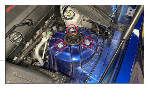
Open the vehicle hood, and locate the (3) 13mm bolts securing the top of the strut to the vehicle. Remove the bolts and remove the strut assembly from the vehicle.
