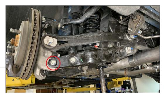
Remove the 15mm bolt retaining the lower control arm to the rear knuckle. Slowly lower the floor jack to lower the control arm while relieving spring tension. Once the spring is relieved of pressure, remove the upper coil spring and isolator from the vehicle. Allow the lower isolator to remain in the control arm.
