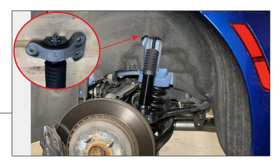
Transfer the shock absorber upper mount from the original shock to the new adjustable shock.
