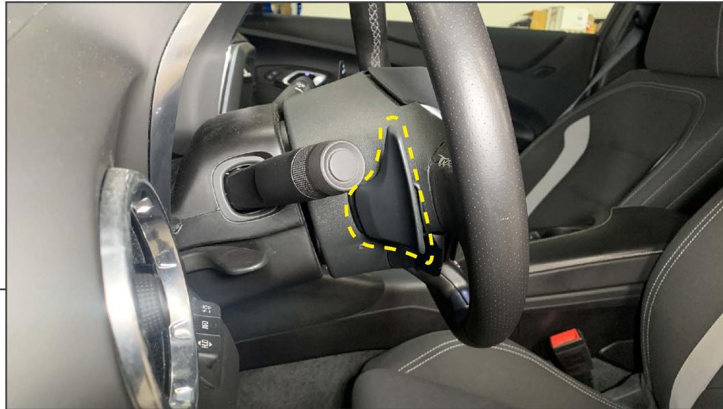
Clean the vehicle paddle shifters using the included alcohol prep pads. Then, clean the paddle shifters using the adhesion promoter prep pads, and allow to fully dry. Once dry, familiarize the fitment of the shifter extensions to the vehicle before removing the tape backing.
