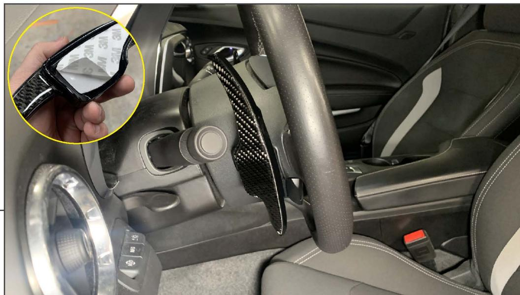
Peel the double sided tape backing, and firmly press the paddle shifter extension to the vehicle paddle shifter. Apply firm pressure to ensure proper adhesion.
