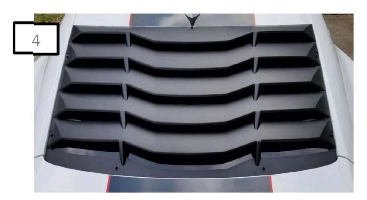
It's good to have a person to help at this point. Lay the louver on the rear window to get a good feel for the way it will fit. Once comfortable, remove the 3M tape backing and carefully lay the louver into place.
