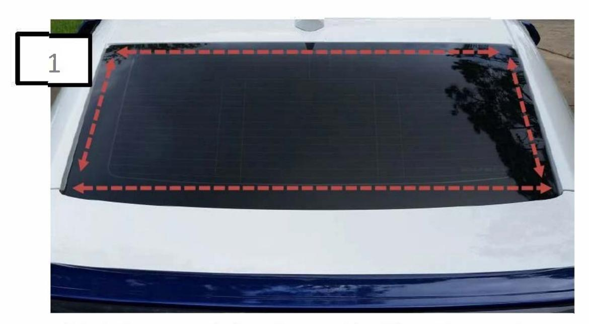
Wash the rear window thoroughly. Allow the area to dry. \*\*Recommended: Wipe the edges of the rear window glass with isopropyl alcohol to ensure the cleanest surface possible.
