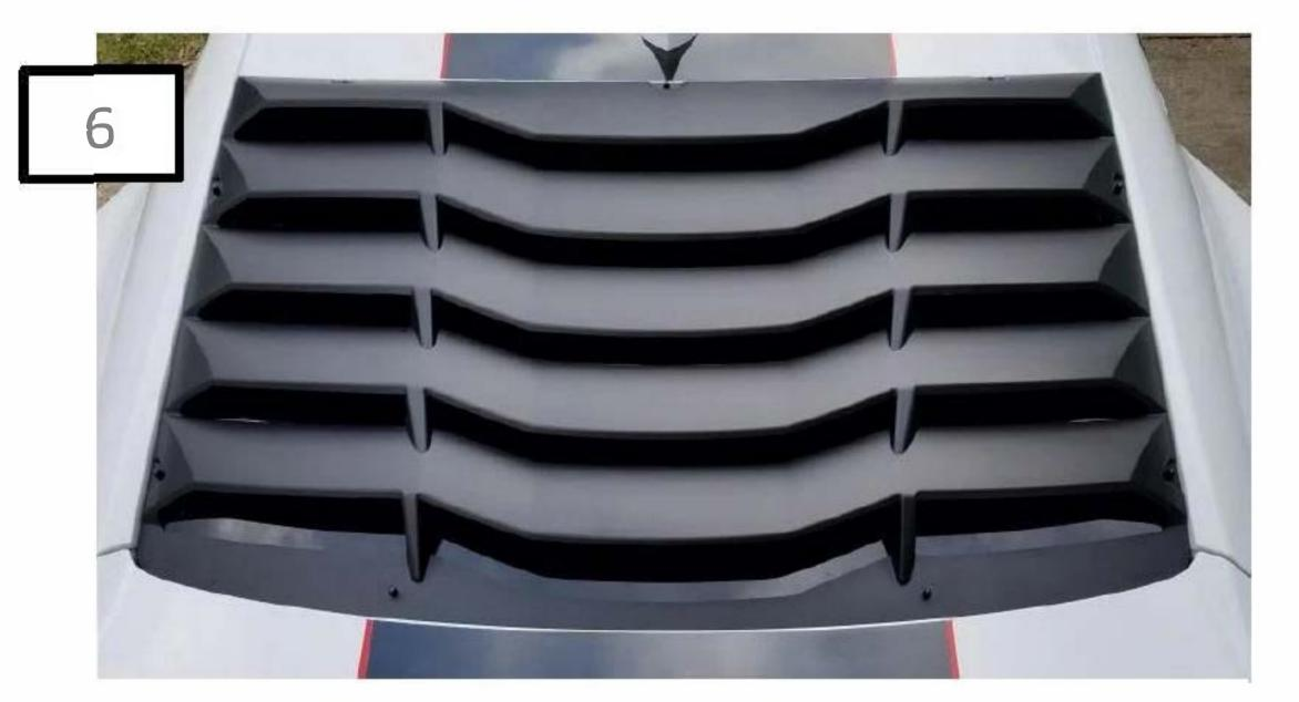
Remove all nuts and remove the louver with brackets still on window. Once again push each bracket firmly into place to ensure good adhesion. Place the louver back into place and tighten the nuts with a 7mm socket. Hand tight is also suitable.
