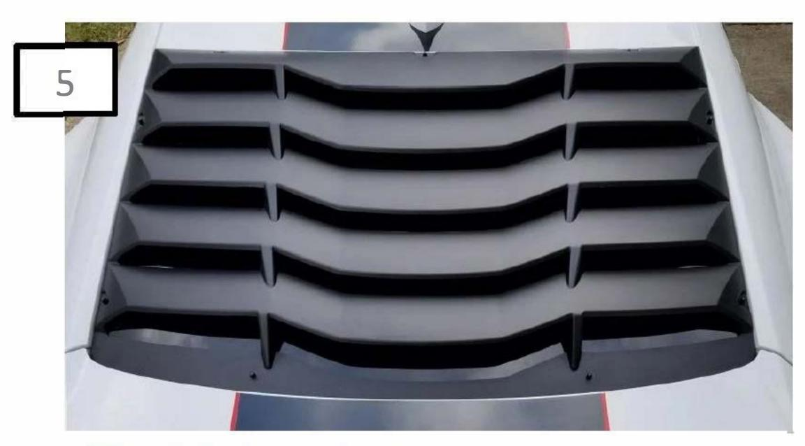
\*\*Watch for sharp edges!! With the louver in place, push all of the metal brackets down firmly. Reach under the louvers as necessary to ensure all brackets are smooth, flush and firmly in place.
