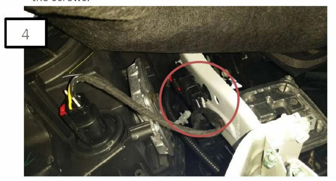
Repeat steps 1-3 for the remaining fender side. When working on the driver's side, be sure to disconnect the large plug.
