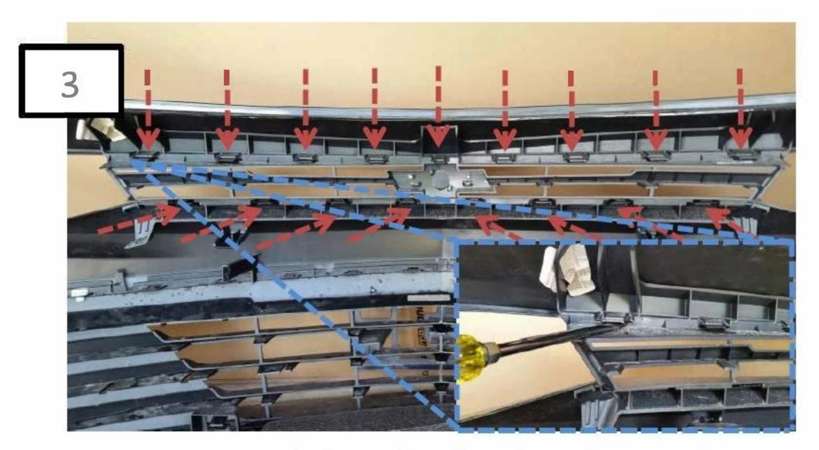
Begin prying each clip and pulling the grille away from the bumper. \*\*Recommended: Starting on either the left or right; Pry the first top and bottom clips, then work your way towards center unsnapping each clip. Do the same for remaining side until grille is free.
