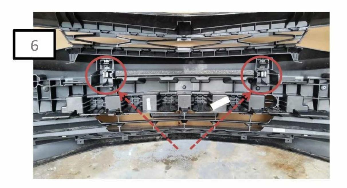
Slide the Styrofoam/Plastic bumper guard back into place and push the two clips firmly back into place.
