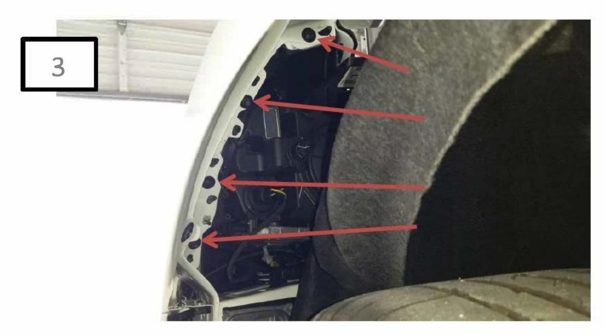
Remove the 4 screws along the fender edge with the 7mm socket.
