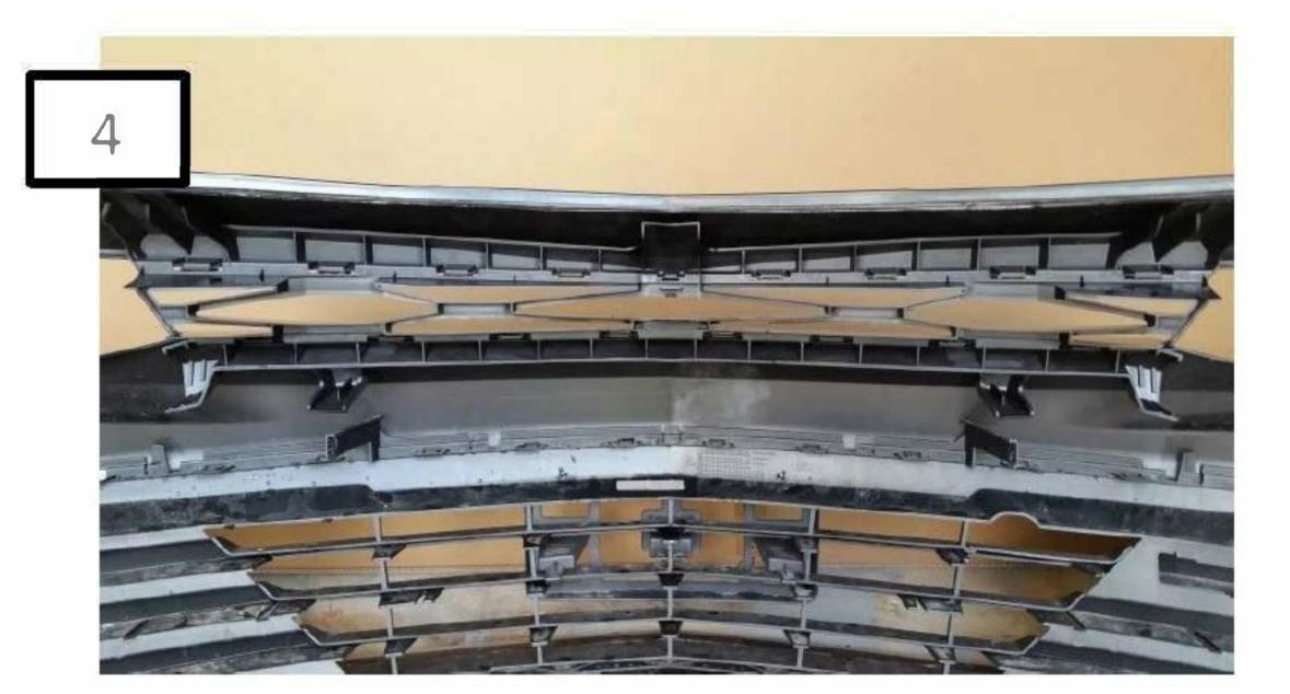
Place the **EXECUTEFTS** grille into place by aligning (not yet snapping) all top and bottom clips.
