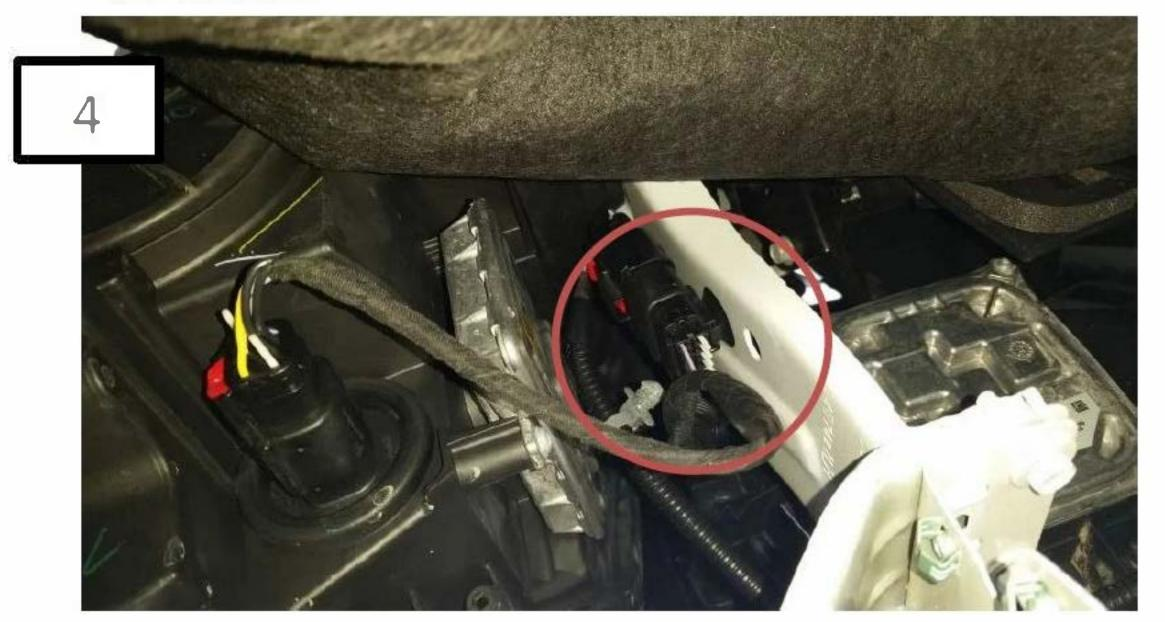
Repeat steps 1-3 for the remaining fender side. When working on the driver's side, be sure to disconnect the large plug.
