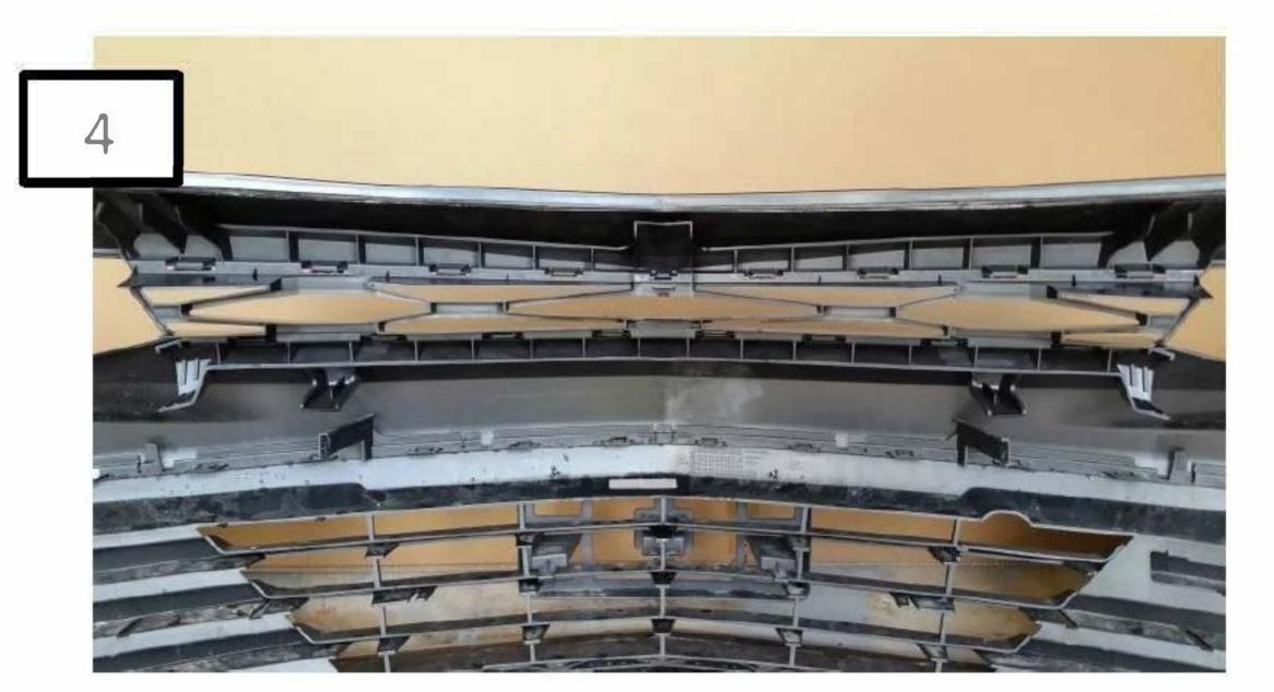
Place the **FIECONCEPTS** grille into place by aligning (not yet snapping) all top and bottom clips.
