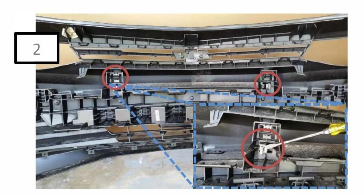
Remove the Styrofoam/Plastic bumper guard by prying off the left and right clips. Pull the guard away and set aside as it will be reinstalled later.
