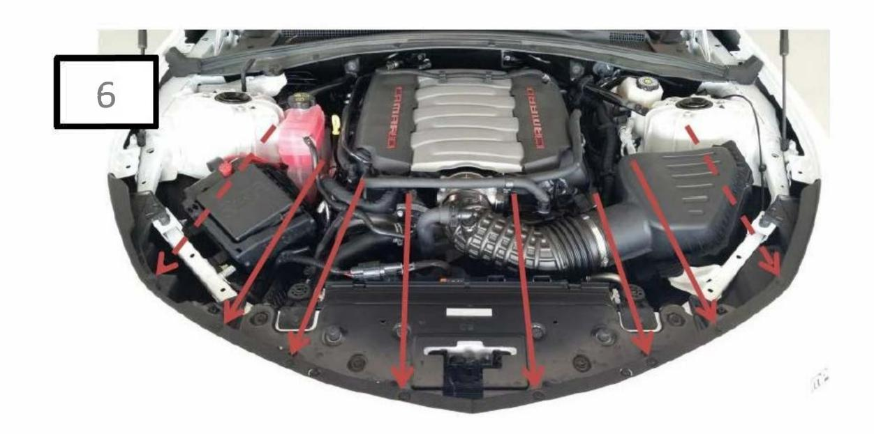
Remove the 6 top screws with a T15 Torx driver.
