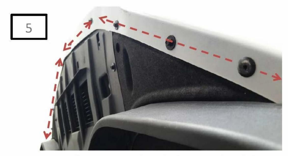
Remove the 12 screws along the bottom edge of the bumper with a 7mm socket. Ignore the 2 torx screws.
