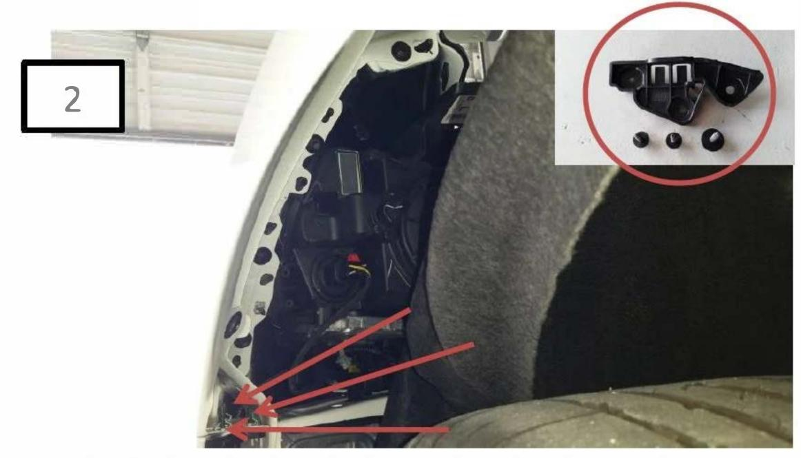
Push the wheel well aside and unplug the parking lamp. Remove the 3 screws with a 7mm socket. Save the plastic insert! \*\*Recommend: Unsnap and remove the parking lamp from bumper to more easily access the screws.
