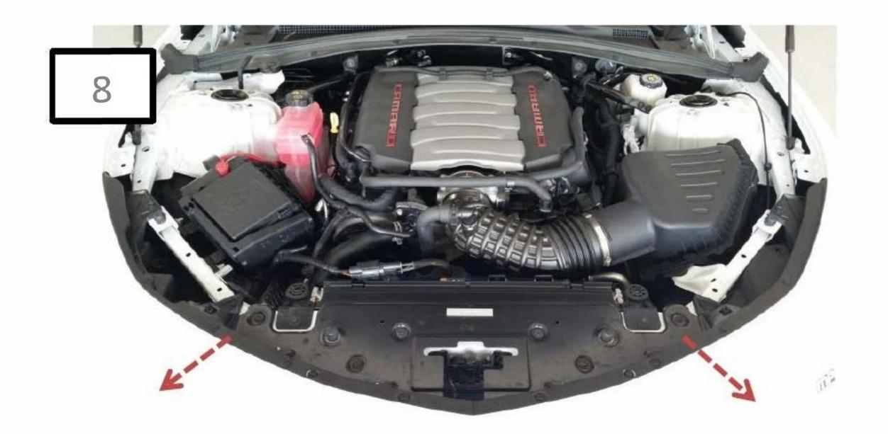
Lift top front edge and begin pulling the bumper away from the vehicle. Bumper removal is now complete.
