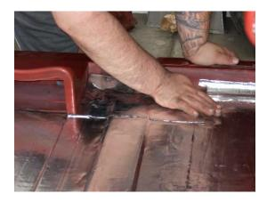
Start at one straight edge (side rail or base of the firewall) and work either side to side or front to back. About the sheet edges or overlap slightly using HushMat's Hush Pro Roller to press down on the material. A single layer of material provides outstanding sound and thermal insulation performance.
