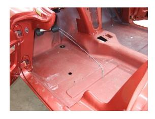
Remove the seats, carpet and trim panel sections surrounding the firewall and tunnel on both driver and passenger side. Remove carpet pad and any loose foam pieces down to the floor pan surface. There no need to remove factory damping material unless it is delaminating or flaking. If it is delaminating or flaking just remove the loose pieces.
