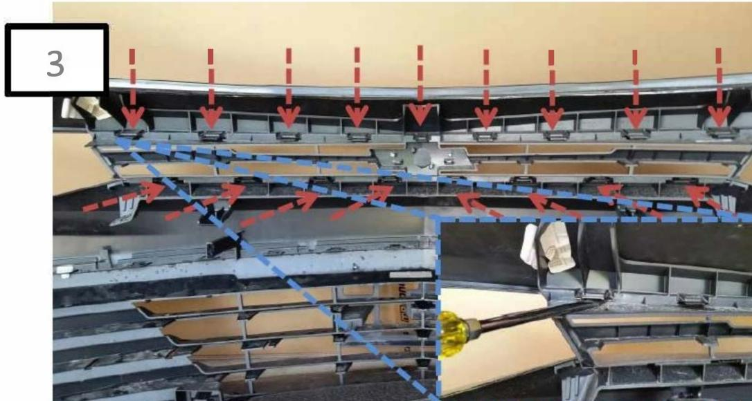
Begin prying each clip and pulling the grille away from the bumper. **\*\***Recommended: Starting on either the left or right; Pry the first top and bottom clips, then work your way towards center unsnapping each clip. Do the same for remaining side until grille is free.
