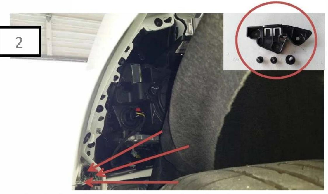
Push the wheel well aside and unplug the parking lamp. Remove the 3 screws with a 7mm socket. Save the plastic insert! **\*\***Recommend: Unsnap and remove the parking lamp from bumper to more easily access the screws.
