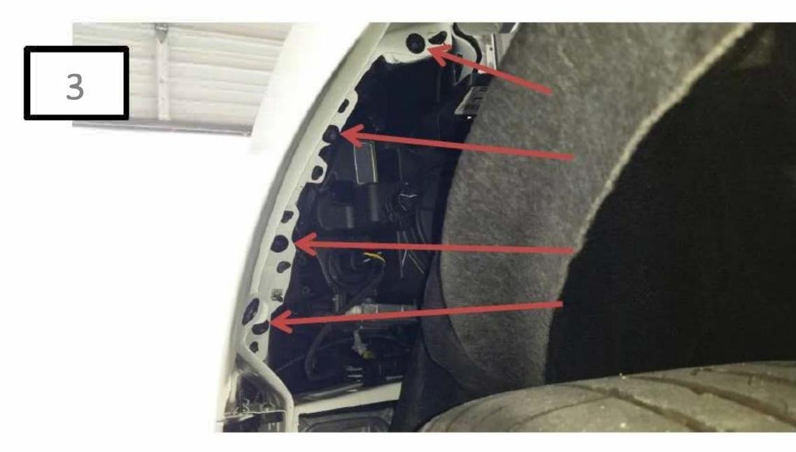
Remove the 4 screws along the fender edge with the 7mm socket.
