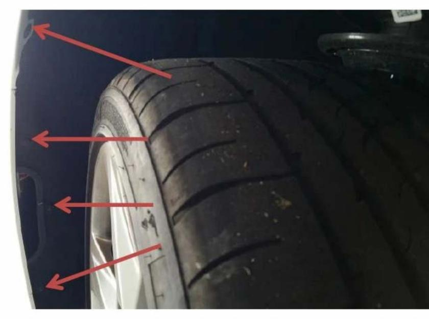
Turn either tire to access the wheel well. Remove the 4 screws with a T15 Torx driver.
