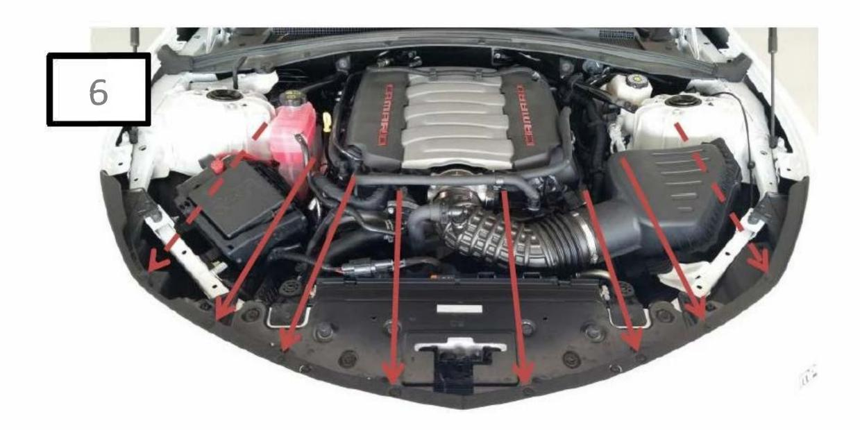
Remove the 6 top screws with a T15 Torx driver. Remove the two push pins on the far left and right. Ignore the 2 screws not marked by arrows.
