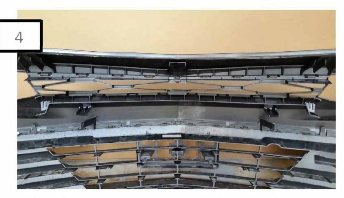
Place the *Internets* grille into place by aligning (not yet snapping) all top and bottom clips. \*\*Recommended: Start with aligning all bottom clips and nearly snapping the far left and right bottom clips. Then align all top clips.
