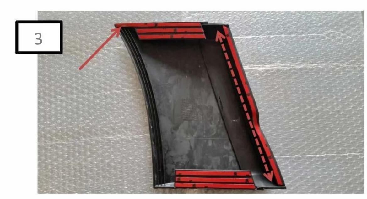
Apply the supplied 3M tape to each side scoop as shown above. Be sure to run tape all the way a crossed the top edge. Align the tape along inside edge of vertical vent to help hide tape edges after scoop installation.
