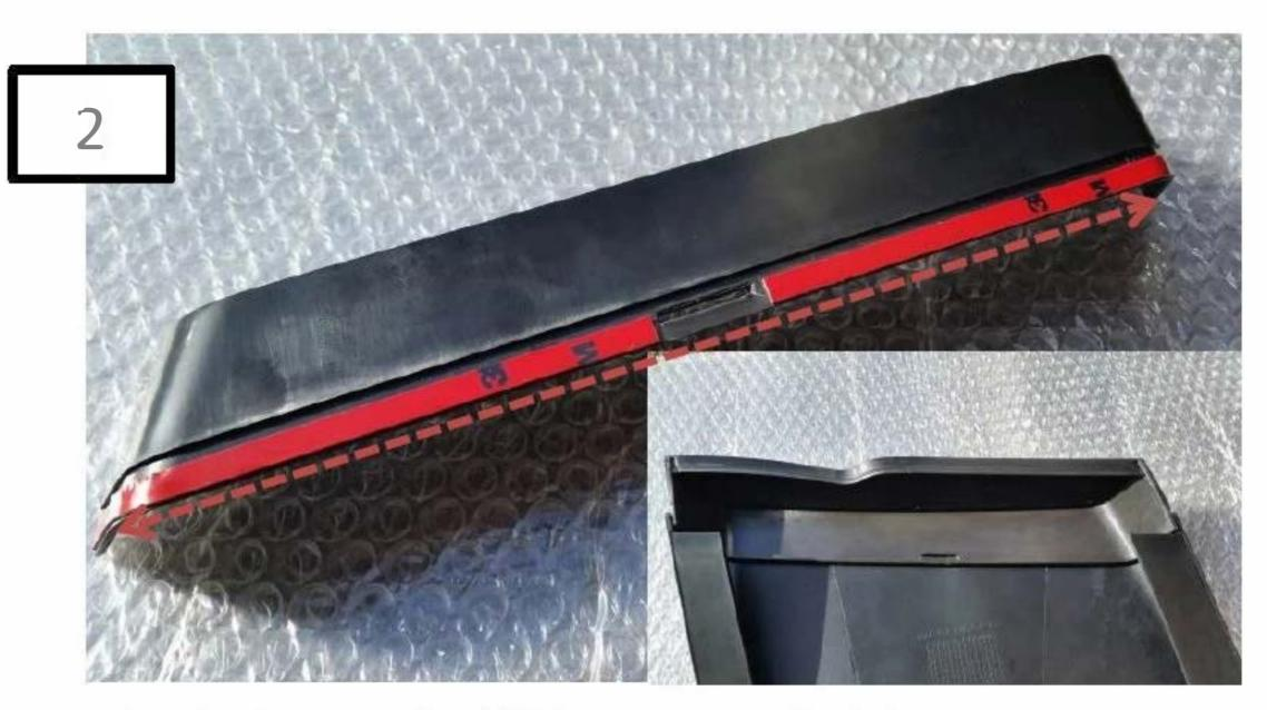
Apply the supplied 3M tape to each side scoop vent (along the inside edge) insert as shown above. Remove the 3M tape backing and push the vent insert firmly into place on each side scoop.
