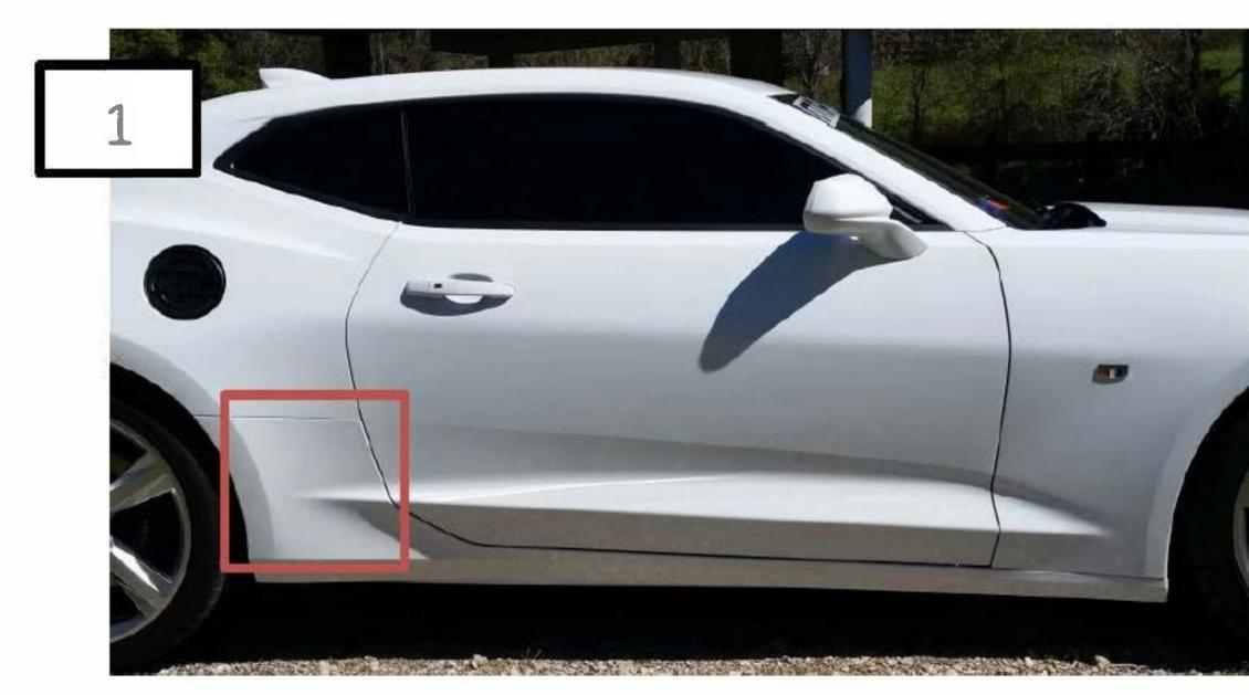
Wash each area with soap and water. Allow the area to dry. \*\*Recommended: Wipe the installation area with isopropyl alcohol to ensure the cleanest surface possible.
