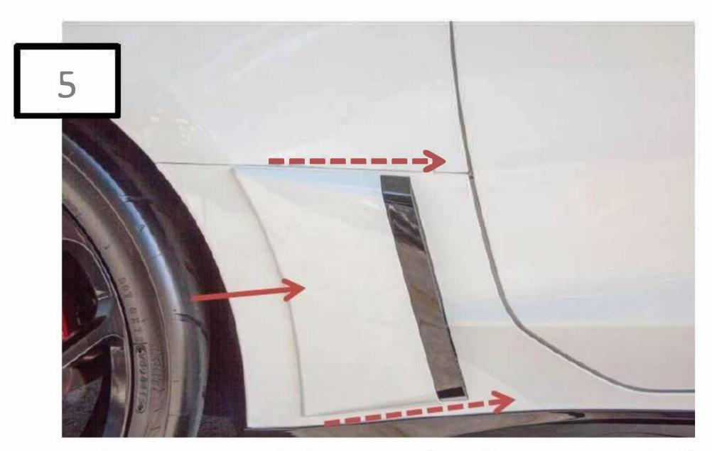
It's recommended to start the placement with the back edges of the side scoop, slowly pushing the whole scoop into place from back to front.
