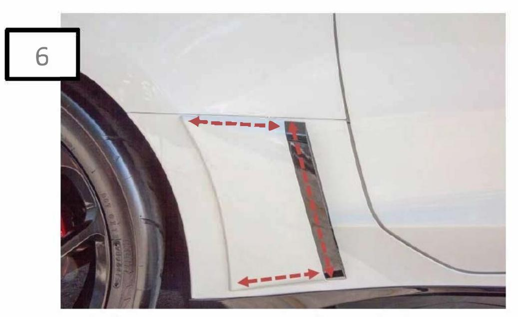
Apply firm even pressure to all taped edges to ensure proper adhesion. Repeat steps 2 through 6 to complete installation of the other scoop.
