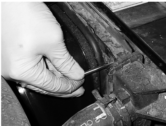
Install temp. probe near inlet hose...
