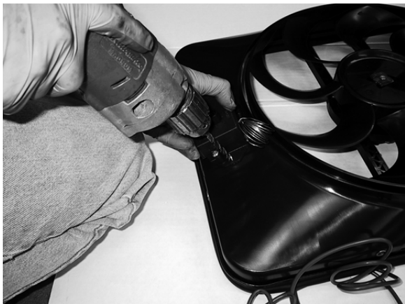
If necessary, drill two \frac{3}{16} " holes...
