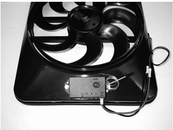
and if mounting control box to the shroud, they can be connected now.
