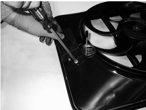
and mount control module in desired location.
