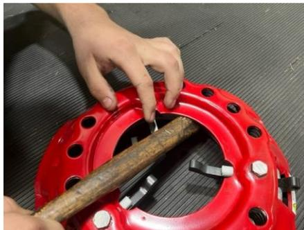
Fig 3 shows lever blocks being removed and the handle letting the lever up. Do this to all three levers and put them in your toolbox or discard them in the trash if you never intend to use them again. Again CAUTION!!! Should be taken not to place your fingers between the lever and the stamped steel cover at any time during this exercise. The handle could slip and catch your finger between the lever and cover incurring injury to or others.
