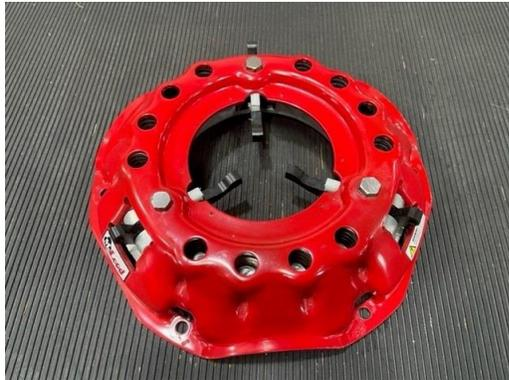
Lever Blocks are used to block down the fingers of the pressure plate, which relieves the stress on the bolts as you tighten them to the flywheel during installation. These blocks MUST be removed after the pressure plate has been installed over the disc and the bolts have been torqued to their final value. Fig 1 shows the three lever blocks installed between the fingers and the pressure plate.
