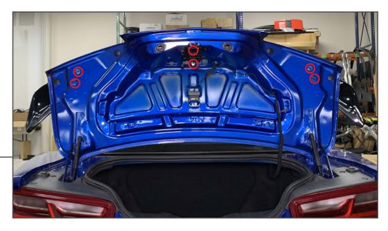
Align the spoiler to the vehicle trunk lid. Secure the spoiler using (6) M6 bolts and (6) M6 flat washers. Ensure to tighten all of the hardware evenly.
