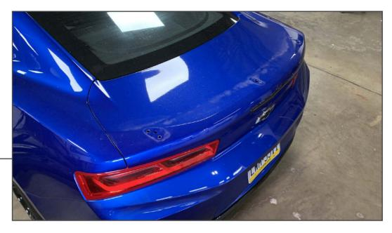
Close the vehicle trunk lid, and use fishing line to seperate the double sided tape in between the original spoiler and the vehicle trunk lid. Clean the vehicle trunk lid with exterior detailer and a microfiber cloth, allow to fully dry.
