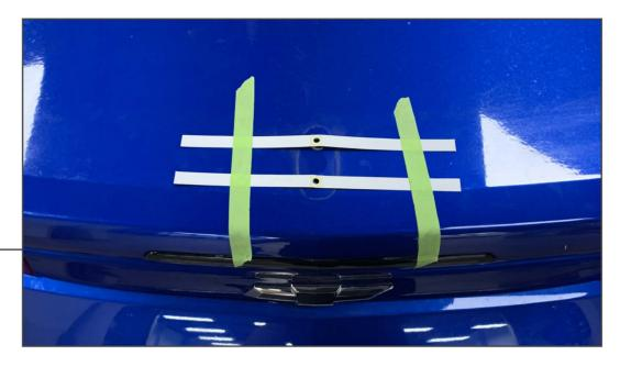
Align and center the spoiler assembly to the rear of the trunk lid. With the drilling templates against the vehicle, secure the drilling templates using masking tape. Remove the drilling templates from the spoiler and set the spoiler aside on a soft surface.
