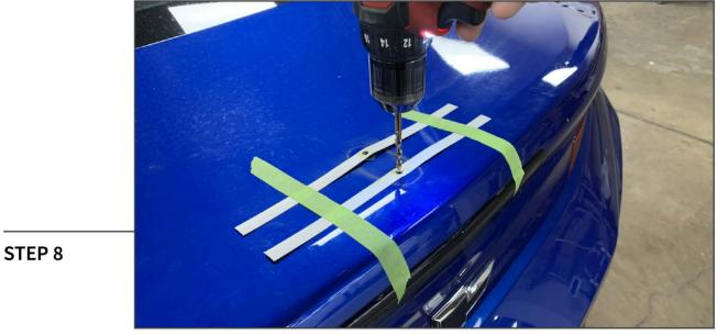
Using a 15/64" drill bit, drill the (6) holes in the vehicle spoiler.
