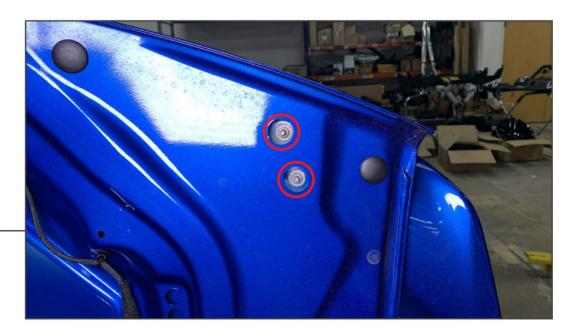
Remove (2) 10mm nuts from each side of the spoiler. With the hardware loose, hinge the trunk lid downwards, then remove the hardware to allow gravity to keep the hardware in the socket.
