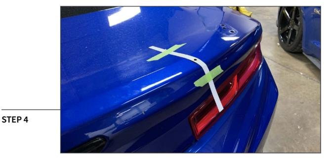
Align and center the spoiler assembly to the rear of the trunk lid. With the drilling templates against the vehicle, secure the drilling templates using masking tape. Remove the drilling templates from the spoiler and set the spoiler aside on a soft surface.
