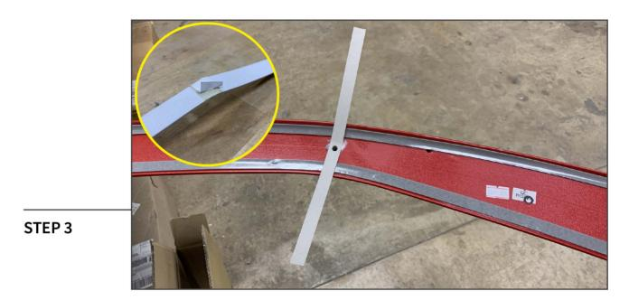
Adhere the drilling templates to the bottom side of the spoiler over the bolt holes.
