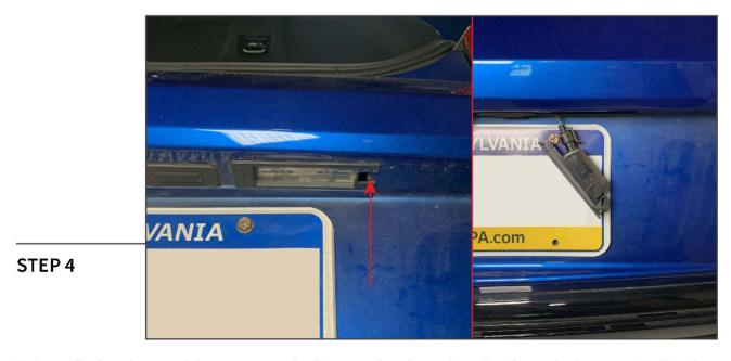
Using a flathead screwdriver, remove the license plate lamp housing from the bumper. Splice the rear diffuser light wiring to each license plate lamp following the diagram below. The lights will power on with the license plate lamps using this diagram.
