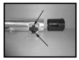
Step 8 Insert and fasten the MAFS onto the Spectre Performance intake tube with the provided machine screws. Insert the MAFS sleeve into the intake tube (note position of slot to allow clearance for the MAFS).
