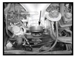
Install the throttle body adapter onto the throttle body.
