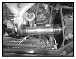
Step 15 Install the 90° coupler with the flex end on the intake tube. Once on the tube, place the other end of the coupler over the throttle body. Once the filter is set in location to clear the reservoir, fasten the couplers in place.
