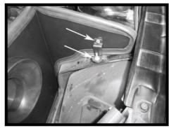
Install the heat shield bracket onto the stud of the inner fender and using the factory nut removed in Step 6, fasten securely. Using the supplied hardware, fasten the bracket to the heat shield.
