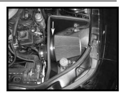
Install the filter on the velocity stack adapter and fasten it securely.
