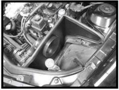
Step 10 Install the heat shield by sliding the heat shield under the lip of the radiator support and in position as shown.
