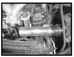
Step 14 Install the Spectre Performance intake tube on the coupler that is on the heat shield with the breather tube pointing towards the motor. Once in position, fasten it securely using the supplied clamp.
