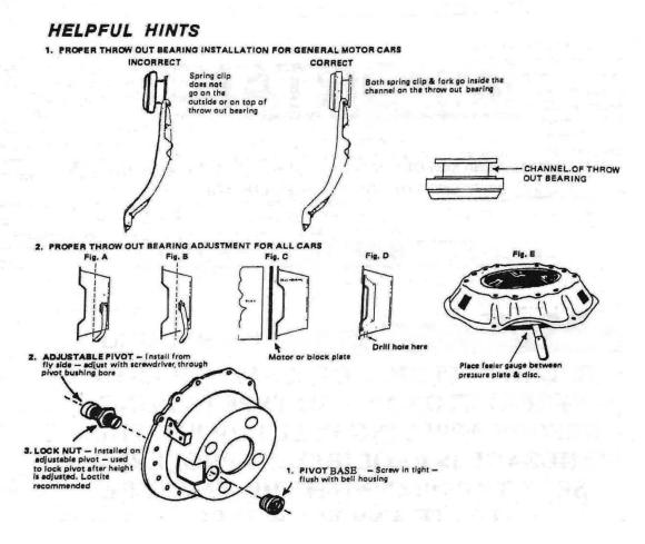
It is very important you follow proper installation procedures during clutch replacement; while second most important is proper adjustment.
