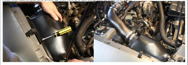
Go back and make any adjustments to the tube and tighten the clamps **(ONLY FINGER TIGHT).** Installation is complete.
