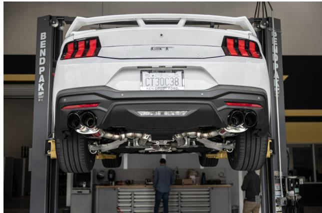
**Step 7.** Once a final position has been chosen for the new exhaust system, evenly tighten all clamps and fasteners, from front to rear, using the torque specifications on page one of the instructions. Inspect all fasteners after 25-50 miles of operation and re-tighten if necessary.
