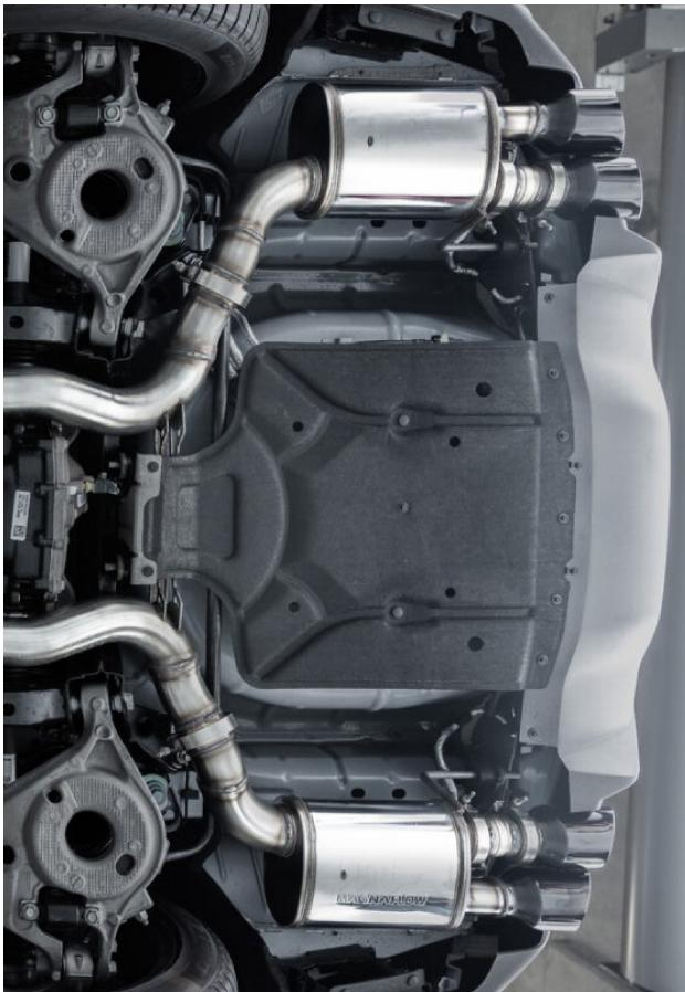
**Step 6.** Next install the passenger side Muffler Assembly followed by the driver side Muffler Assembly using supplied V clamps and engaging the hangers into the rubber insulators. Finish the installation by loosely attaching the MagnaFlow bracket between the Extension Pipes. Re-attach the valve wiring for the valves and make sure they are secured properly away from the heat of the mufflers.
