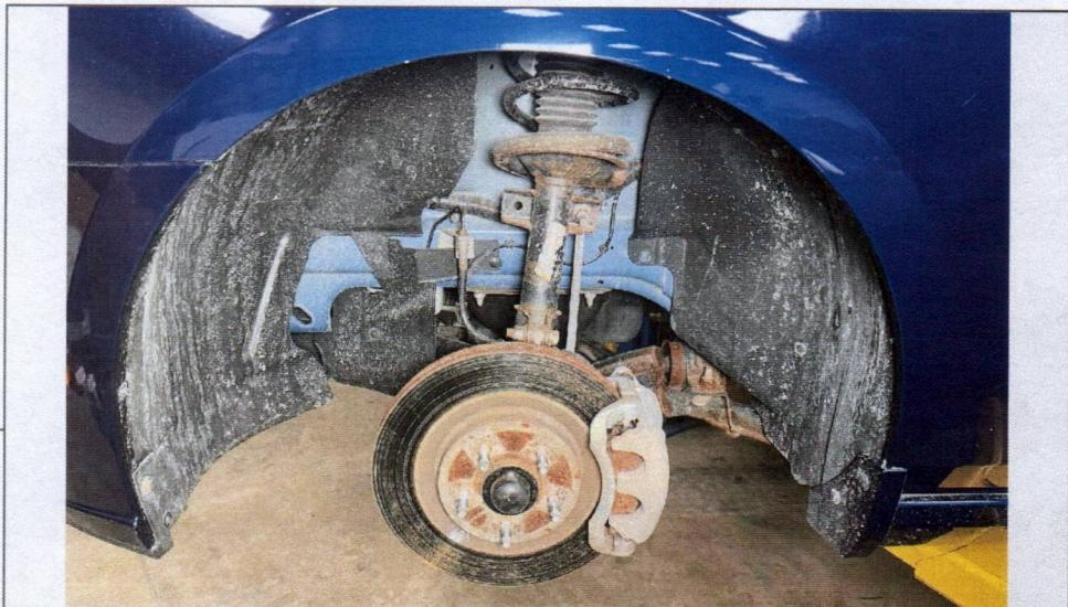
Safely lift and support the front of the vehicle using a floor jack and jack stands. Remove the front wheel from the vehicle to access the suspension components.
