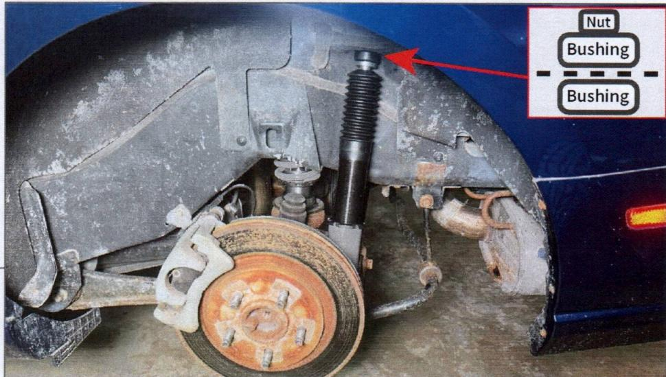
Fit the top of the new shock absorber through the vehicle body. Then, loosely install the top of the shock absorber to the body through the trunk using (1) rubber bushing and (1) flange nut included with the shock absorber.
