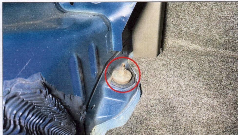
Open the vehicle trunk, and remove the trunk liners by removing various plastic clips. Then, remove the upper shock absorber nuts to remove each shock absorber from the body.
