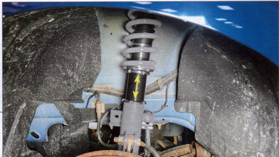
To adjust ride height, loosen the lower collar and turn the coilover assembly up/down to adjust the ride height.
