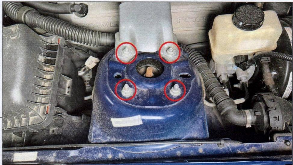
Open the vehicle hood. Remove the (4) 13mm nuts securing the top of the shock absorber to the strut tower.
