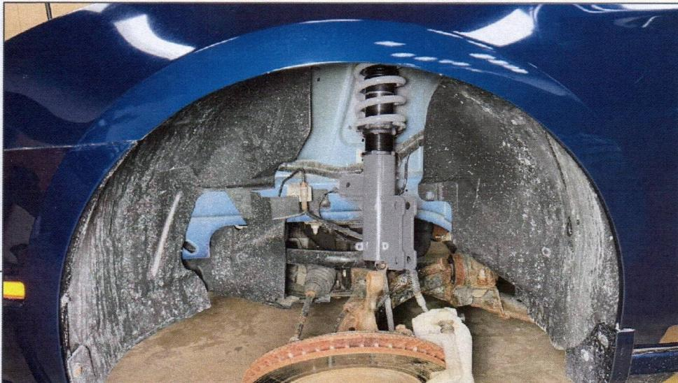
Fit the top of the coilover assembly into the strut tower holes, and loosely secure using the included (4) flange nuts.
