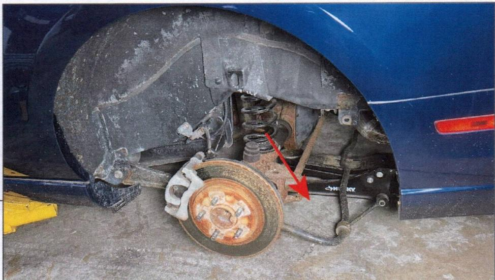
Lower the floor jack to allow the rear axle to lower from the vehicle. Remove the coil springs from the rear axle. Allow the upper and lower spring isolators to remain in the vehicle.
