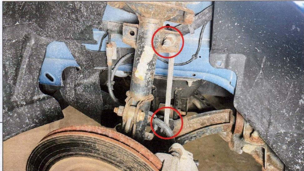
Remove the (2) 18mm nuts securing the sway bar link to the shock absorber and the sway bar, and remove from the vehicle. If the sway bar link joint spins when loosening the nut, hold the joint using a 8mm socket and use a wrench to loosen the nut.
