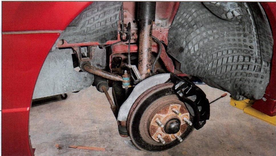
Safely lift and support the vehicle off the ground. Remove the vehicle wheels. Identify the suspension components.
