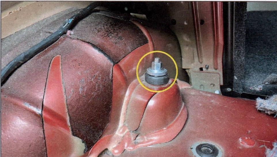
Open the trunk, and remove the trunk liners to reveal the upper shock mount. Remove (1) 15mm nut securing the top of the shock absorber to the shock tower in the vehicle trunk.
