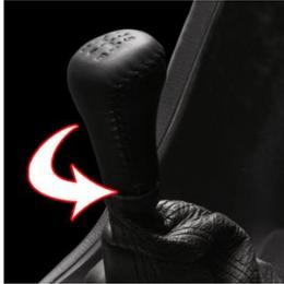
1. Remove the factory shift knob by simply unscrewing it counter-clockwise.
