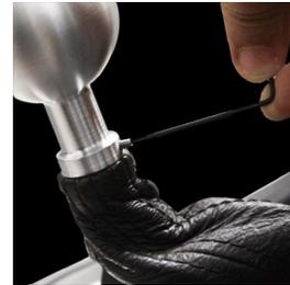
2. Install the new shift knob to the desired location and lock in place with supplied set screw and allen key.
