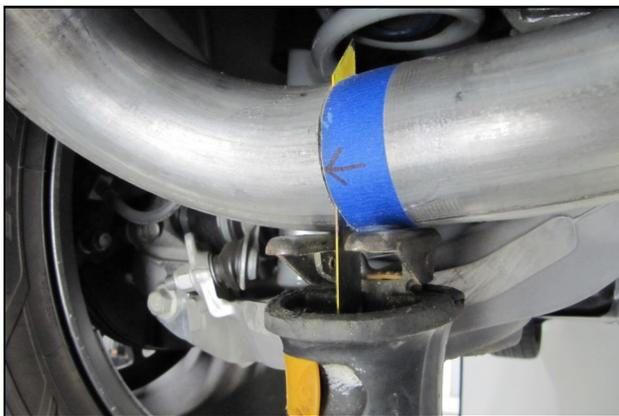
**3.** With the help of an assistant to brace the muffler, cut the OEM exhaust system using a Sawzall® or equivalent.
