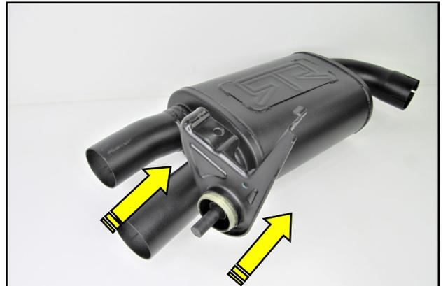
**8.** Reinstall the OEM exhaust hanger onto the RTR Muffler as shown, with the white half of the bushing facing rearward.
