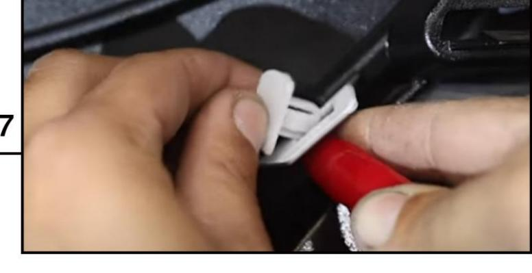
Depress the locking tabs on the retainer clips and slide them towards the center of the grill to remove them, then remove the OEM grille from the bumper cover. Align the bumper cover tabs with the slots in the new grille to install it. Reinstall the retaining clips into the center of the bumper cover. Press the OEM harness anchors into the slots in the side of the new grill. Reinstall the energy absorber and reattach the multi-pin connector.
