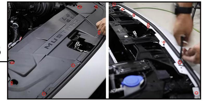
Remove the 8 plastic rivets in the core support cover and remove the cover from the vehicle. Use a 7 mm socket to remove the 5 screws along the upper bumper cover. Carefully remove the weather strip foam from the cleat in the core support on both sides of the vehicle. Lift the bumper cover up and over the core support posts and remove the cover.
