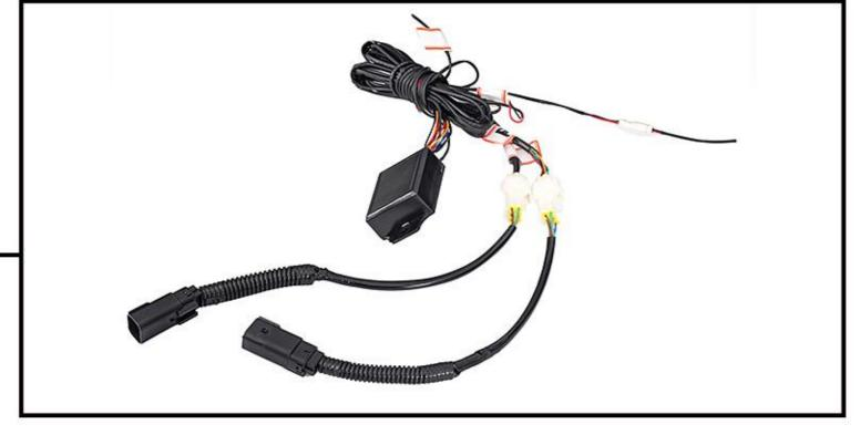
(1) Connect the new grille light plugs to the OEM grille light wiring harness; Note: Connect the "L" plug to the driver side OEM grille light wiring harness; Connect the "R" plug to the passenger side OEM grille light harness.(2) Connect the red wire to ACC; the black wire to the negative terminal of the battery.
