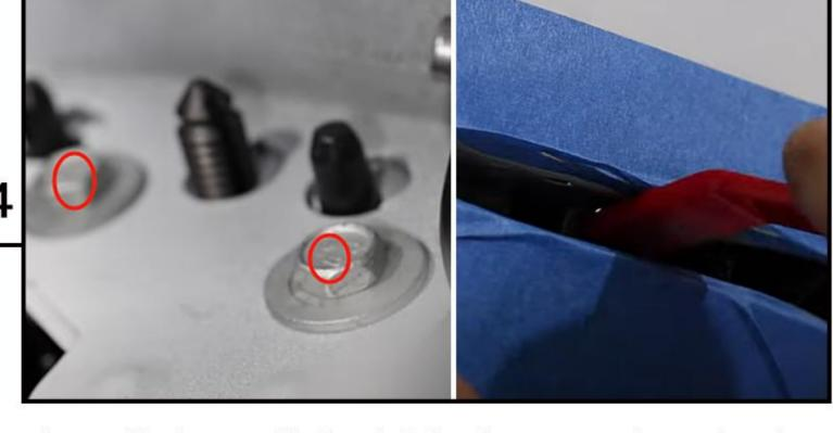
Behind the headlights will find 2 bolts securing the bumper corner, remove the 2 bolts with a 10 mm socket and repeat the step on the opposite side of the vehicle. Pry the fur tree anchors out from the fenders with a panel clip removal tool after applying a little painter tape.
