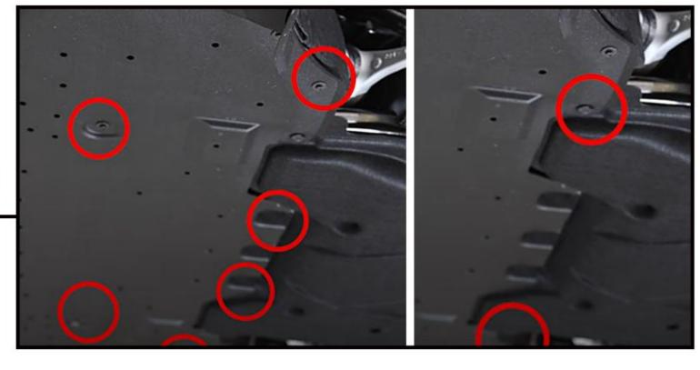
Remove these 6 screws in the debris shield underneath the car with a 7mm socket. Then pride the center post out of these 2 plastic rivets and remove. STEP 2
