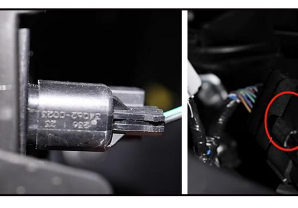
With the fender liner pulled back, locate and disconnect the side marker lights inside the bumper cover. Then locate and disconnect the bumper wiring harness on the driver's side of the car which is attached to the crash pad.
