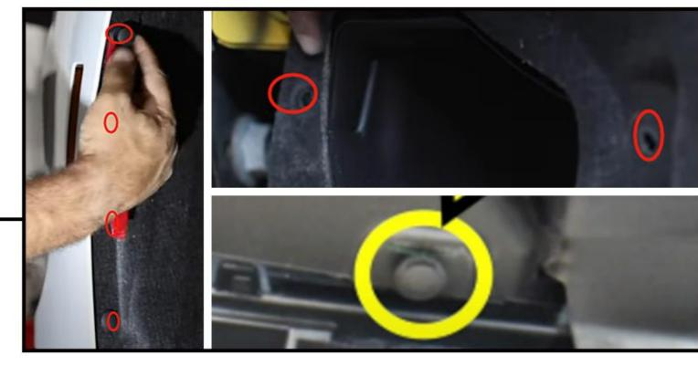
Remove the four plastic rivets from both of the fender liners. For performance pack cars, remove the four plastic rivets from both the fender liners followed by removing these 2 small rivets in the brake cooling Ducks, then remove the single plastic rivet in the cooling duck inlet to lower grille and remove them from the vehicle.
