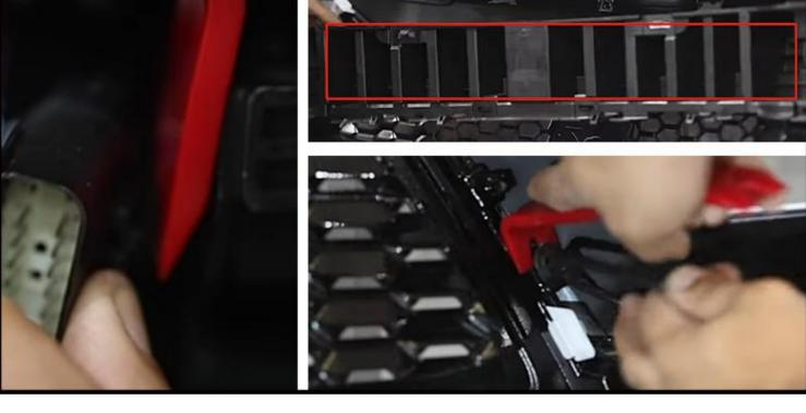
Pry the large multi-pin connector from energy absorber with a panel clip removal tool. Pull the energy absorber from the bumper with light pressure. Locate and disconnect the OEM grill lights on both side of the grille. Pry the light harness anchors out of the both sides of the upper grille with a panel clip removal tool. Then use the 7 mm socket to remove the 2 screws securing the lights to the grille and remove the lights.
