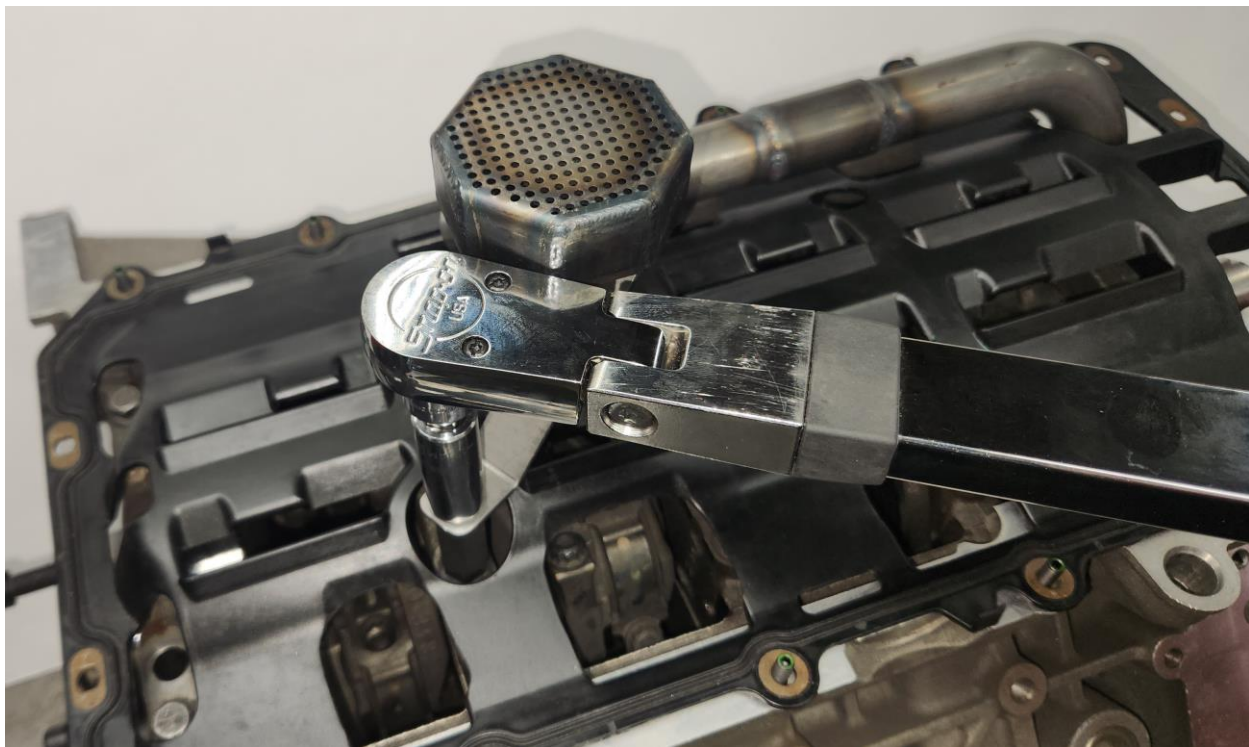
Step 9: Complete installation by torquing the 8mm flange head screw to 25 N-m.
