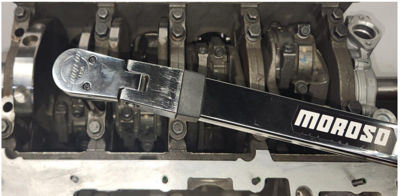
Step 3: Torque the main cap bolt to 65 N-m for the first pass and 90° for the final pass This fastener must be the Moroso supplied bolt for final installation
