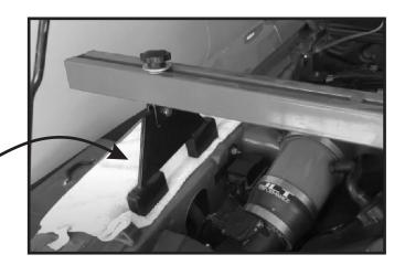
**IMPORTANT**- new mounts may lift engine once installed - check
