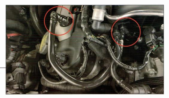
Locate the PCV hard-line circled above. Rotate the gray clip and pull the fittings away from the intake manifold and valve cover.
