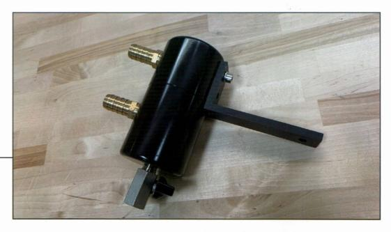
Install the 2 hole mounting bracket using the M6 Allen bolt and washer secure the catch can to the mounting bracket.
