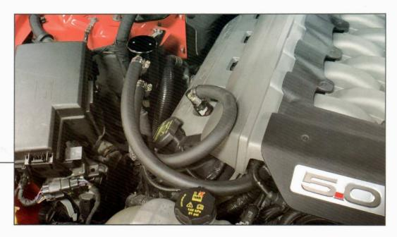
The top fitting on the catch can attaches to the intake manifold. The bottom fitting attaches to the valve cover. Cut the provided hose in half and then route the hose from the catch can to the fittings to the engine fittings. Secure the hose using the provided hose clamps. If necessary, trim the engine cover to fit. Reinstall the engine cover to complete. Drain catch can as needed.
