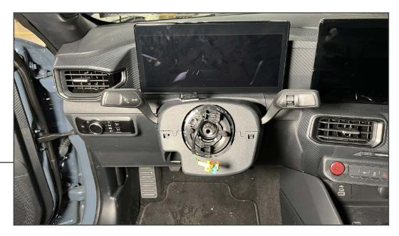
Firmly move the steering wheel to disengage the wheel from the steering column. While removing the steering wheel, carefully route the clock-spring wiring harness out of the steering wheel. Ensure the clock-spring remains in the original position. If the clock-spring moves slightly during steering wheel removal, gently move back to the original starting position.
