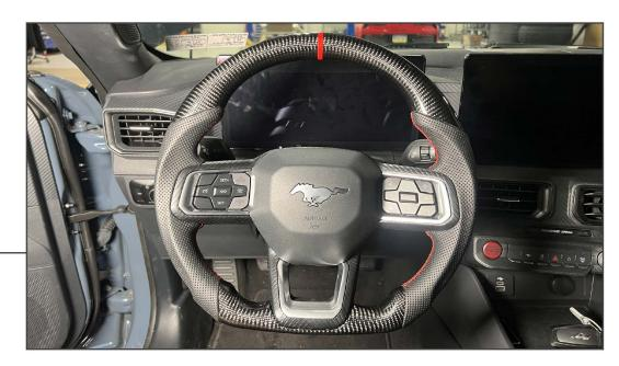
Plug in the three air bag connectors, and press the air bag into the steering wheel until fully seated, the air bag will audibly click into place.
