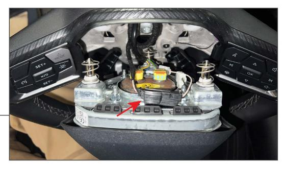
With the air bag removed from the steering wheel, unplug the upper-most connector by pressing the tab and pulling the connector away. The tab is along the back of the air bag, a small pry tool may be necessary to properly press the tab.
