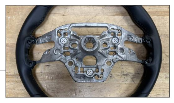
Locate the air bag retaining springs and white retaining clips. Using a flathead screwdriver, remove the spring from the steering wheel. With the spring removed, the white clip will fall out of the steering wheel.
