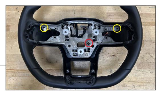
Remove (1) T-20 Torx screw the steering wheel harness ground lead.
