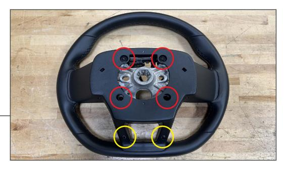
Begin to disassemble the steering wheel by removing (4) T-15 Torx screws from the center of the steering wheel.
