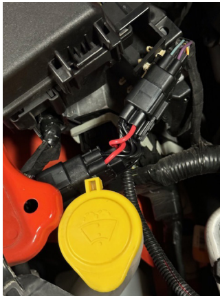
Plug Connectors Together with New Harness
