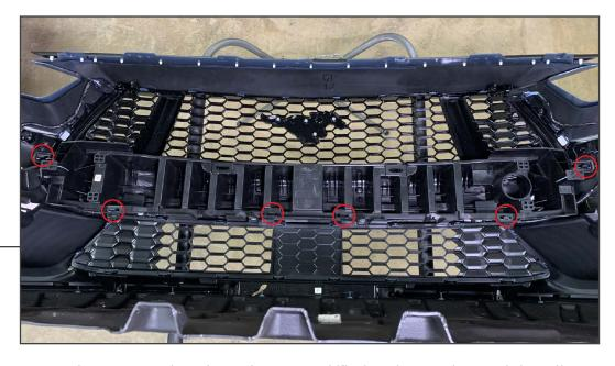
Remove the bumper core by pressing the tabs with a pry tool/flathead screwdriver while pulling the core away.
