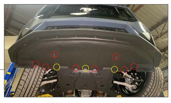
From under the vehicle, remove (8) 7mm screws and (3) plastic push clips to separate the plastic shield from the vehicle chassis.
