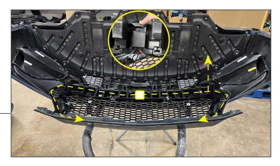
Using the included double sided tape, secure the included wiring harness module to the inside of the bumper core. Then, route the harness along the vehicle grille light harness towards each grille light. Plug in all light connectors and adapter harnesses, and secure the harness into place using the included cable ties. Fit the bumper core to the bumper.
