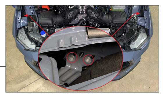
Remove (2) 10mm bolts from each side of the vehicle disconnecting the bumper from the fenders.
