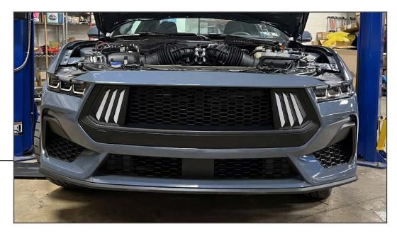
Fit the bumper to the vehicle, and plug in each of the grille lighting harnesses, and each side marker into the bumper lighting.
