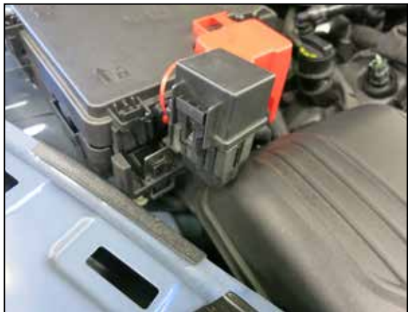
7. Pull back the relay from the fuse box assembly and set aside to allow clearance for air filter housing removal.
