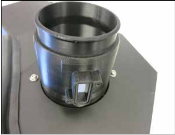
9. Install the K&N MAF housing into the driver side K&N heat shield and secure with the provided hardware.
