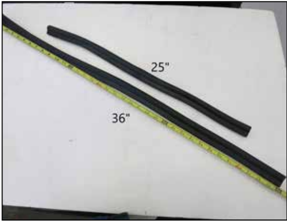
11. Cut the longer 61" edge trim to lengths of 25" and 36".
