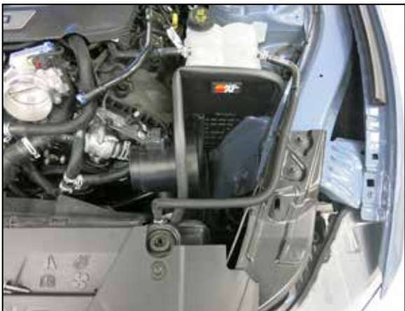
14. Install the heat shield assembly into the driver side so the mounting stud inserts into the factory mounting grommet, then secure with the factory air filter housing mounting bolt removed in step #3.
