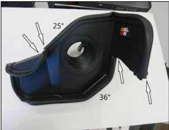
12. Install the cut sections of edge trim onto the heat shield as shown. Install the K&N badge into the heat shield and lock in place from the back side with the provided locking plate.
