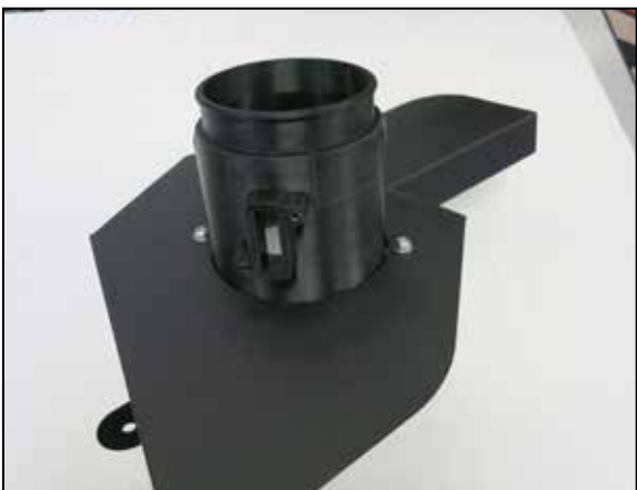
15. Install the remaining K&N MAF housing into the passenger side K&N heat shield and secure with the provided hardware.
