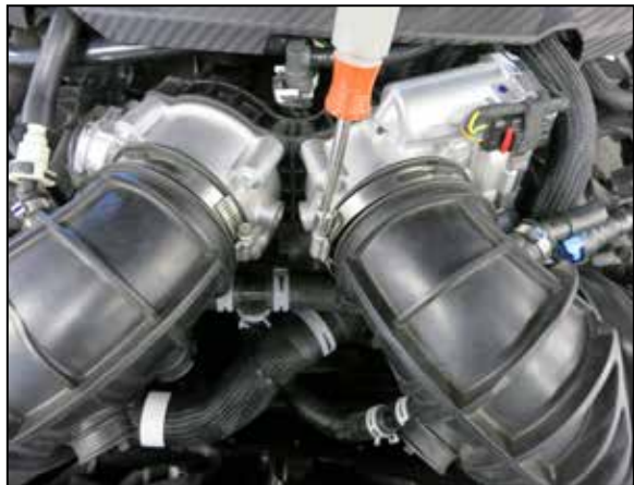
4. Loosen the hose clamp that secures the driver side intake tube to the throttle body. Disconnect the intake tube from the throttle body, lift the air filter housing to dislodge it from the mounting grommet and then remove the complete driver side intake system.
