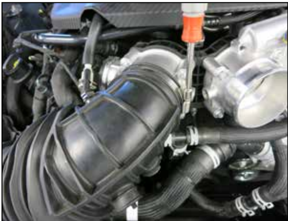
8. Loosen the hose clamp that secures the passenger side intake tube to the throttle body. Disconnect the intake tube from the throttle body, lift the air filter housing to dislodge it from the mounting grommet and then remove the complete passenger side intake system.
