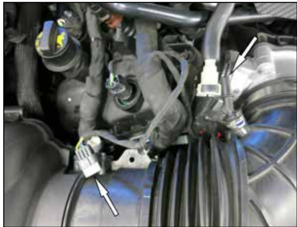
5. Release the locking tab and then disconnect the EVAP hose quick connect fitting from the passenger side intake tube. Release the locking clip and then disconnect the passenger side MAF electrical connection.
