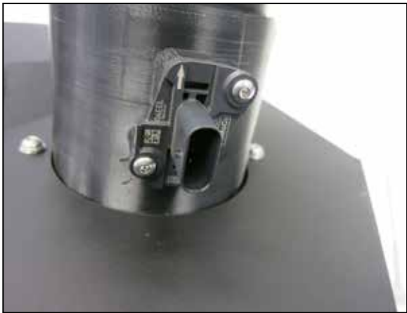
10. Remove the mass air sensor from the factory driver side maf housing and install it into the K&N driver side housing using the provided hardware.
