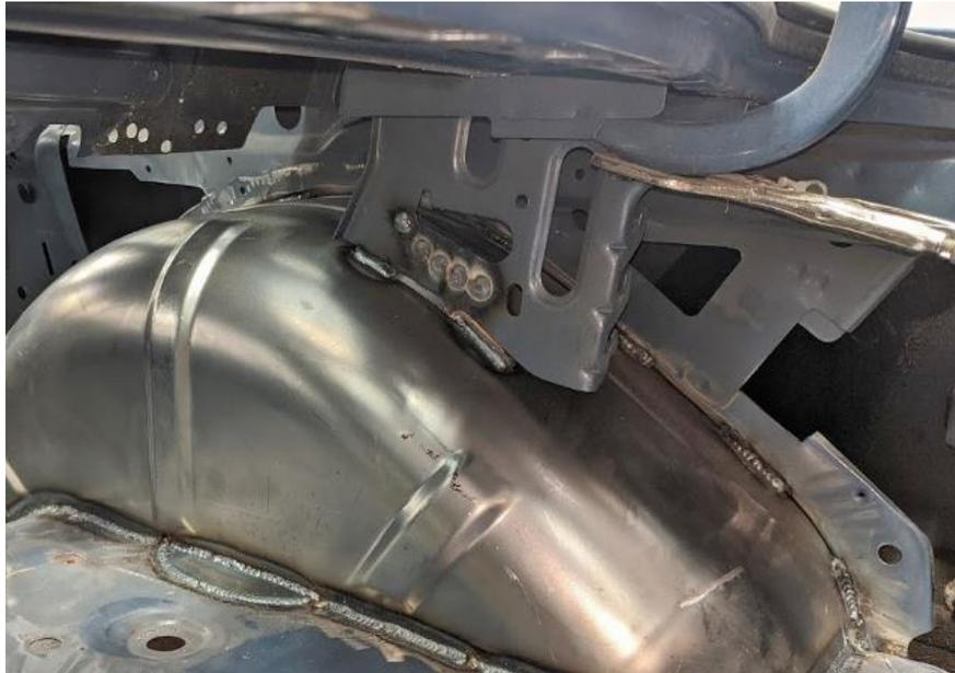
Figure 51 – Re-attach Trunk Hinge Bracket
