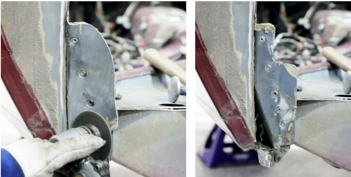
Figure 30 – Remove Inner Wheel Tub Layer
