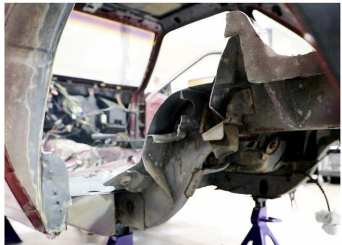
Figure 19 – Remove Front Factory Structure
