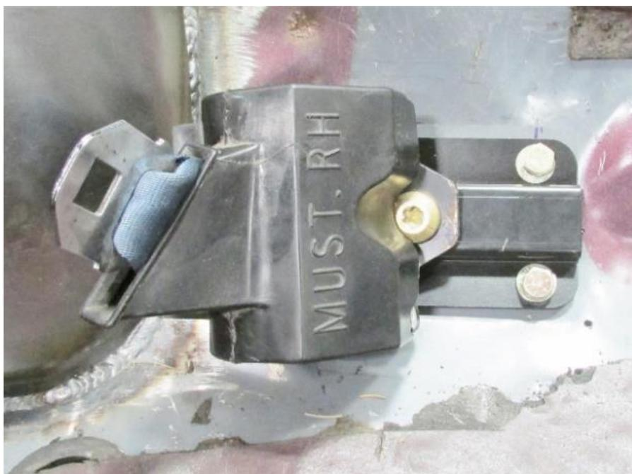
Figure 50 - Torque Seat Belt Assembly
