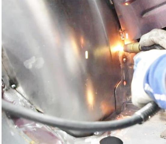
Figure 40 – Tack Weld Flange
