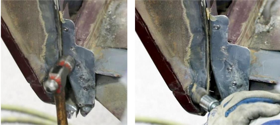
Figure 31 – Adjust Flange
