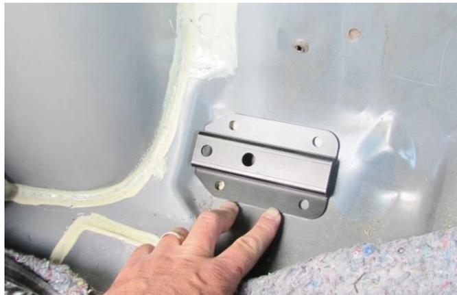
Figure 44 – Seat Belt Relocation Bracket
