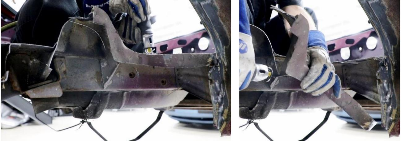
Figure 20 - Remove Rear Factory Structure
