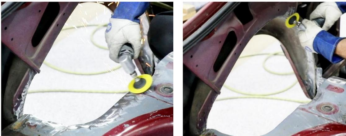
Figure 32 – Grind Sheet Metal
