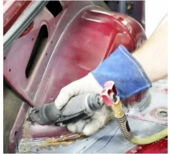
Figure 17 – Cutout Inner Wheel Tub
