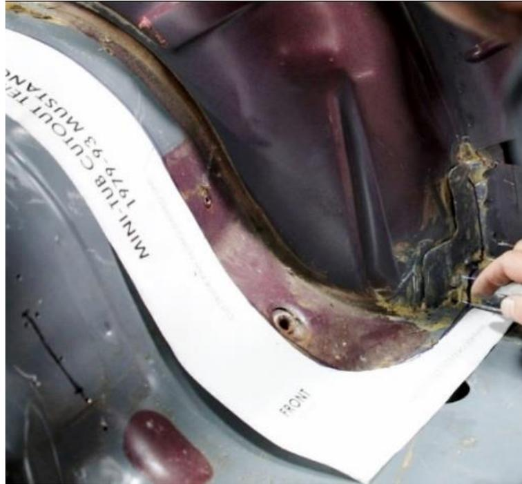
Figure 15 – Locate Front Template
