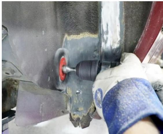
Figure 10 - Locate Spot Welds
