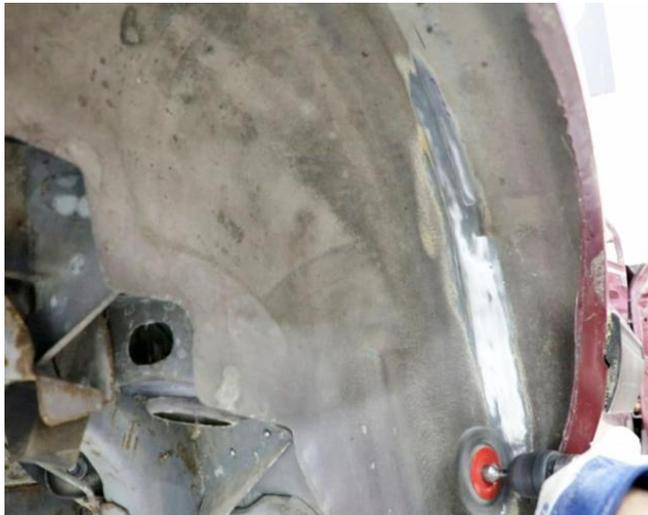
**Figure 8 - Remove Undercoating**
