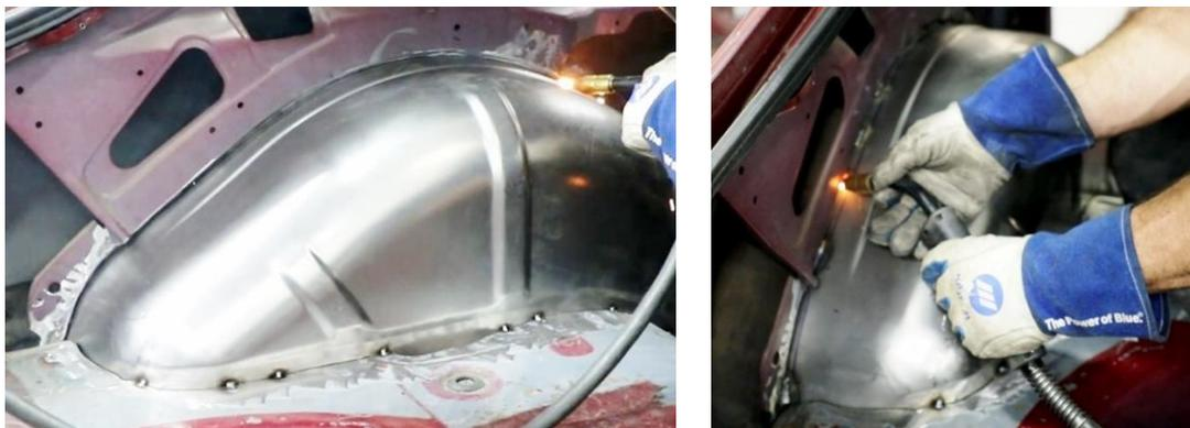
Figure 39 - Tack Weld Mini-Tub
