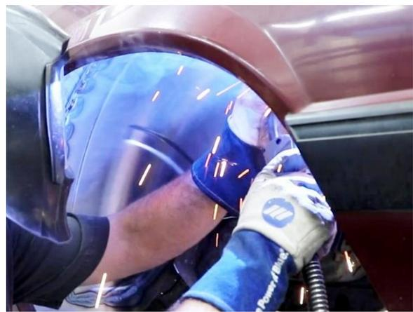
Figure 41 – Finish Weld around Mini-Tub
