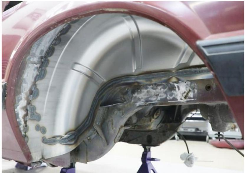
Figure 52 – Mini-Tub Install
