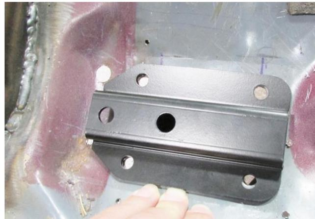
Figure 47 - Drill Bracket Mounting Holes
