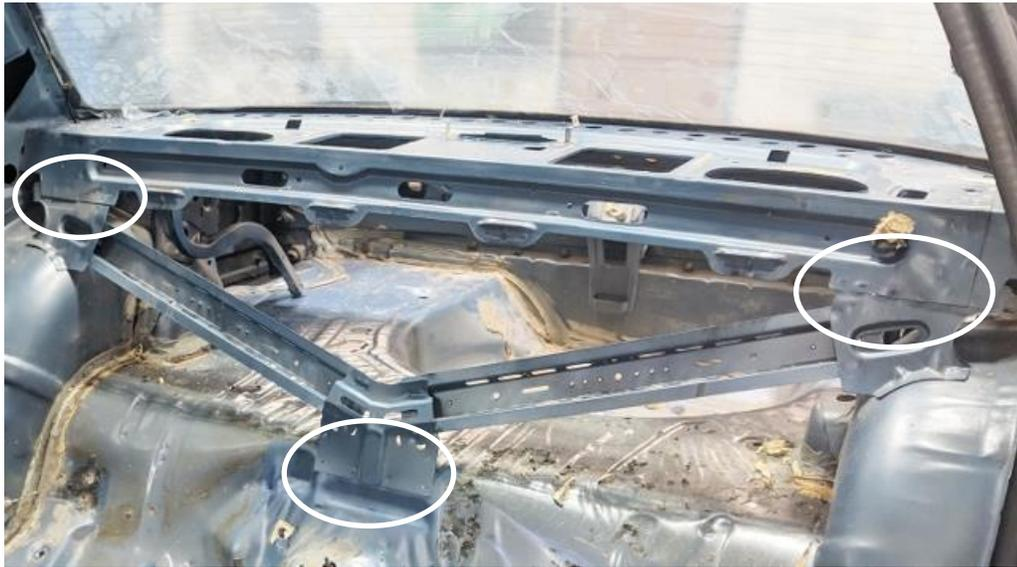
**Figure 3 - Remove Wheel Tub Brackets**
