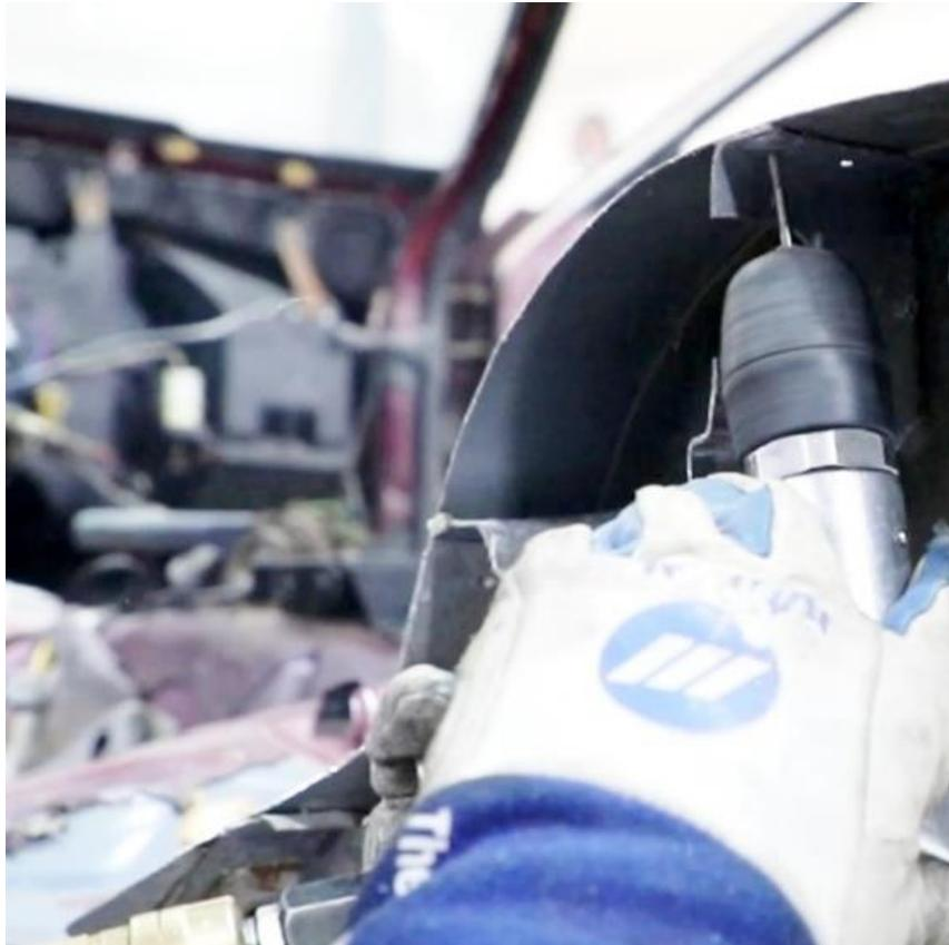
Figure 26 – Remove Spring Perch Spot Welds
