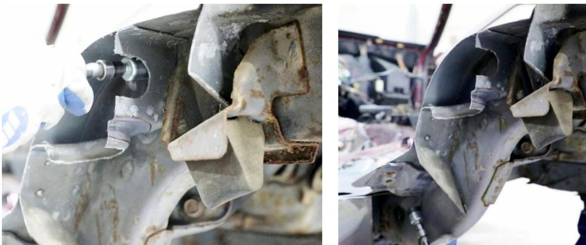
Figure 22 - Expose Spot Welds
