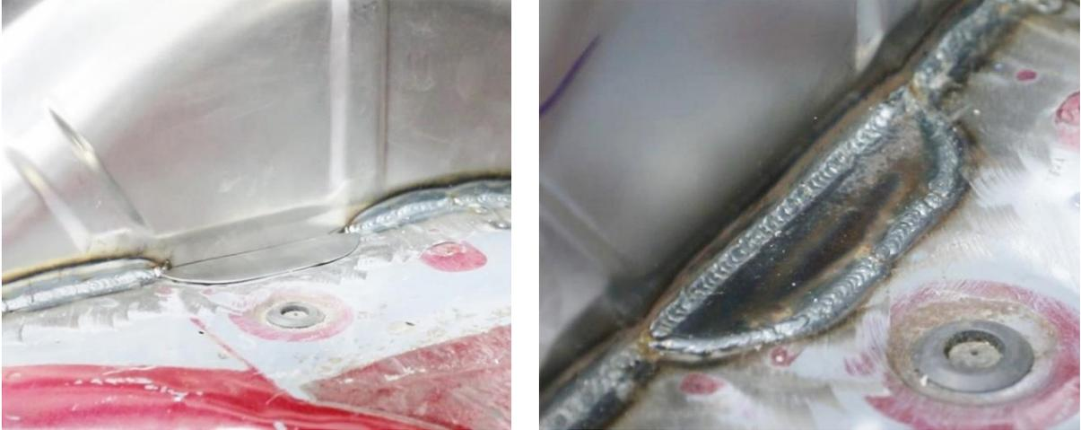
Figure 43 – Weld Closeout
