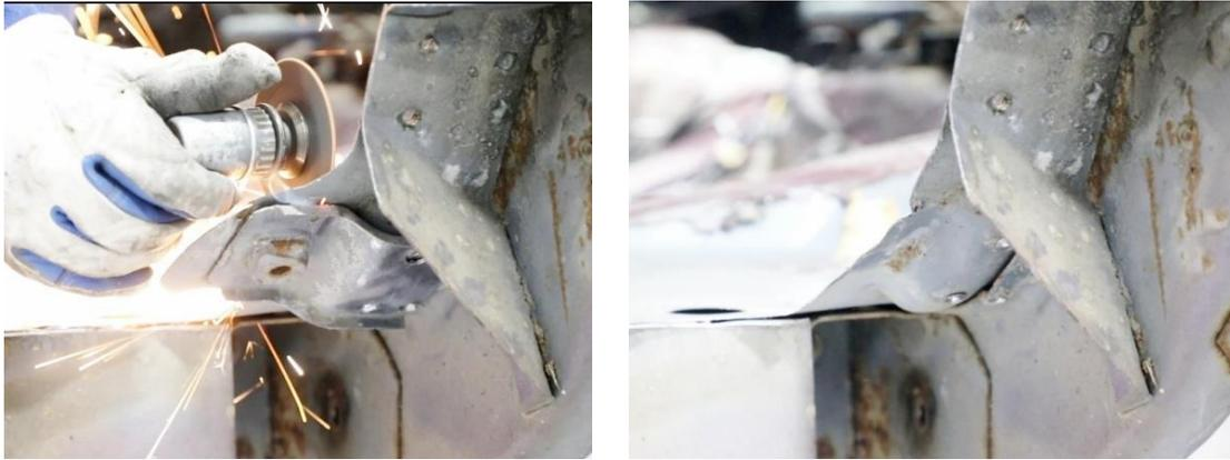
Figure 28 – Remove Seat Belt Anchor
