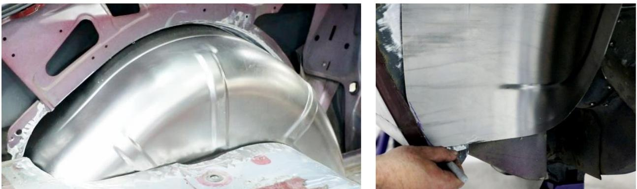
Figure 33 – Test Fit Mini-Tub
