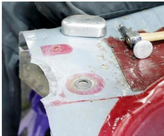
Figure 29 – Flatten Trunk Floor
