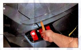
Using a plastic pry tool and a heat gun, heat the spoiler edges to loosen the adhesive and gently pry upwards to disengage the spoiler tape adhesive from the trunk lid. Ensure to protect the vehicle painted surfaces while carefully prying the spoiler away.
