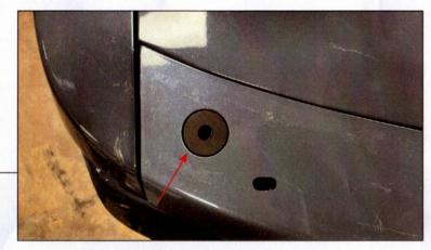
Fit (1) spacer into each of the spoiler mounting points on the trunk lid.
