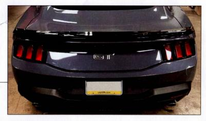
With the tape backing removed, firmly press the spoiler to the vehicle trunk lid to encourage adhesion. Tighten the M5 bolts to secure the sides of the spoiler. Re-install the trunk lid rubber grommets removed in Step 1.
