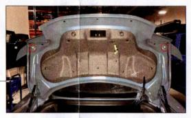
Open the vehicle trunk. Remove (1) rubber grommet from each end of the trunk lid covering the spoiler mounting hardware.
