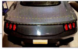
Clean the vehicle trunk lid using exterior detailer and a microfiber cloth. Then, clean the outer perimeter of the trunk lid using (1) alcohol prep pad, followed by (1) adhesion promoter prep pad.
