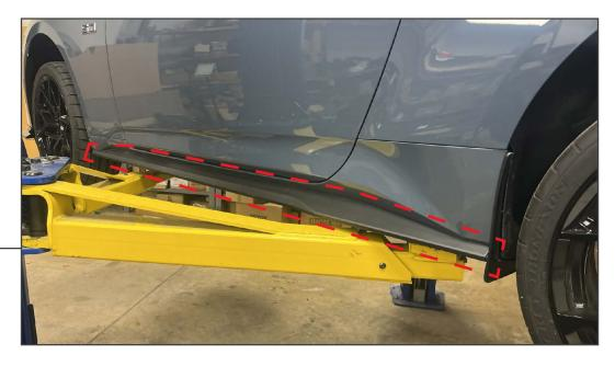
Safely lift and support the side of the vehicle from the ground to access the top and bottom of the OEM side skirt.
