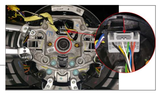
Remove the wiring harness by depressing the clip and pull the plug away from the steering column. Using a 24mm socket, remove the nut securing the steering wheel to the vehicle. Once the nut is removed, firmly hold both sides of the steering wheel and rock it side to side, this will release the wheel from the steering column.
