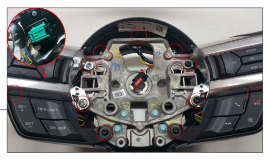
Locate, and remove the T20 torx bit screws securing the controls to the factory steering wheel. Unplug, and remove the controls from the steering wheel. Transfer to the new steering wheel.
