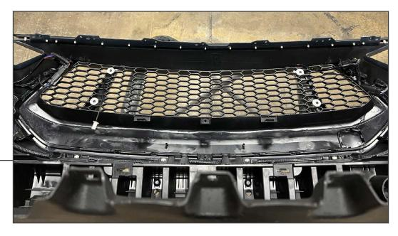
Press the new grille into the vehicle bumper. Ensure all mounting tabs align before firmly pressing into place. Once properly fitted, install the (6) white retaining clips to secure into place.
