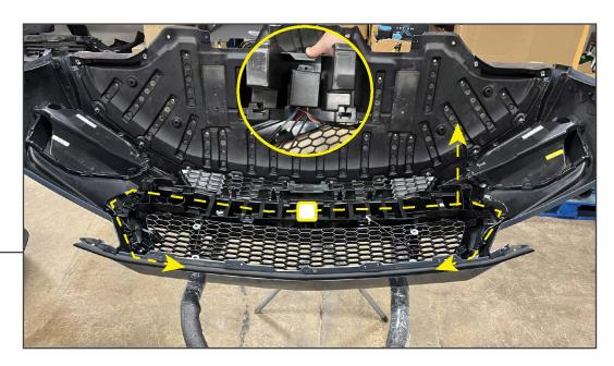
Using the included double sided tape, secure the included wiring harness module to the inside of the bumper core. Then, route the harness along the vehicle grille light harness towards each grille light. Plug in all light connectors, and secure the harness into place using the included cable ties. Fit the bumper core to the bumper.
