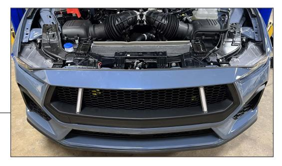
Fit the bumper to the vehicle, and plug in each of the grille lighting harnesses, and each side marker into the bumper lighting.
