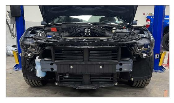
With assistance, lift the top edge of the bumper over the chassis retainer and remove the bumper from the vehicle and onto a soft workable surface.
