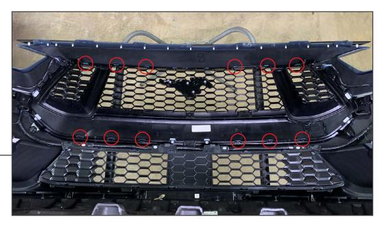
Use a pry tool/flathead screwdriver to press the retaining tabs while pulling the grille away from the bumper. Once all clips are dislodged, remove the grille from the bumper and set aside.
