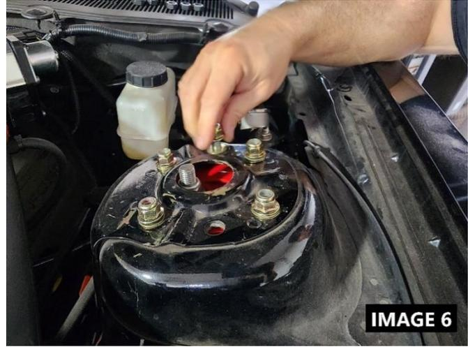
10. Push the studs through the holes in the strut tower and install the nuts and washers on the top. **IMAGE 6**
