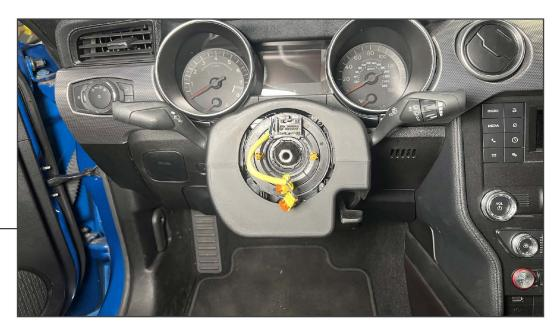
Firmly move the steering wheel to disengage the wheel from the steering column. While removing the steering wheel, carefully route the clockspring wiring harness out of the steering wheel. Ensure the clockspring remains in the original position. If the clockspring moves slightly during steering wheel removal, gently move back to the original starting position.
