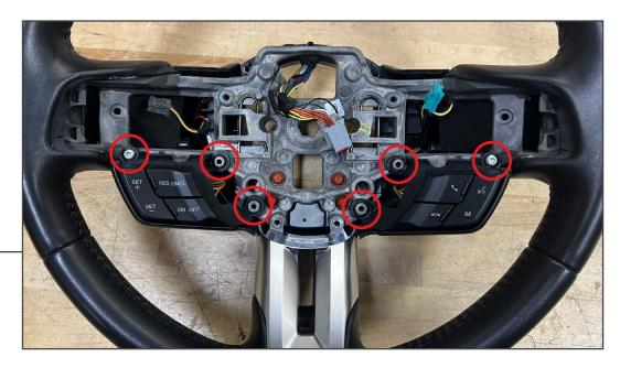
Remove (6) T-20 Torx screws from the cruise control and hands-free switch assemblies.
