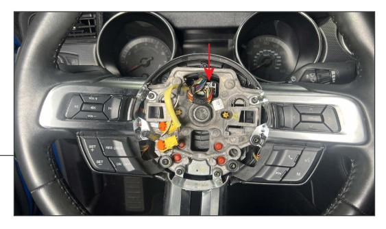
Unplug the steering wheel controls connector by pressing the tab and pulling the connector away.
