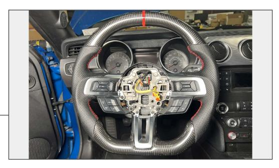
Align the steering wheel to the vehicle, and route the clockspring harness through the steering wheel. Fit the steering wheel to the steering column and secure into place using the original 15/16" bolt.
