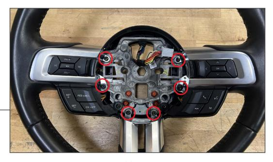
Begin to disassemble the steering wheel by removing (6) T-20 Torx screws from the volume controls, 4-way directional buttons, and the lower trim panel.
