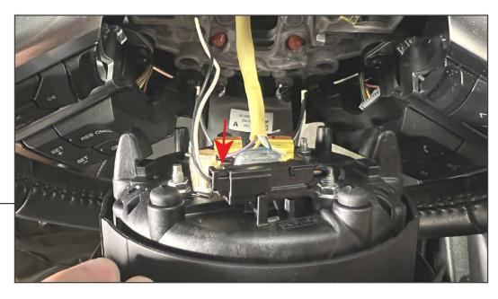
With the air bag removed from the steering wheel, unplug the upper-most connector by pressing the tab and pulling the connector away.
