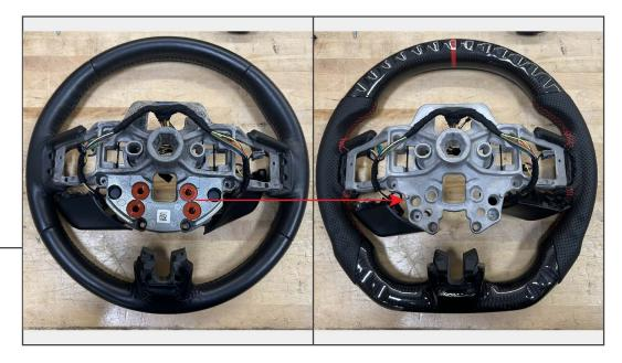
Identify and familiarize the routing of the steering wheel wiring harness. This is important to ensure the harness is transferred properly.
