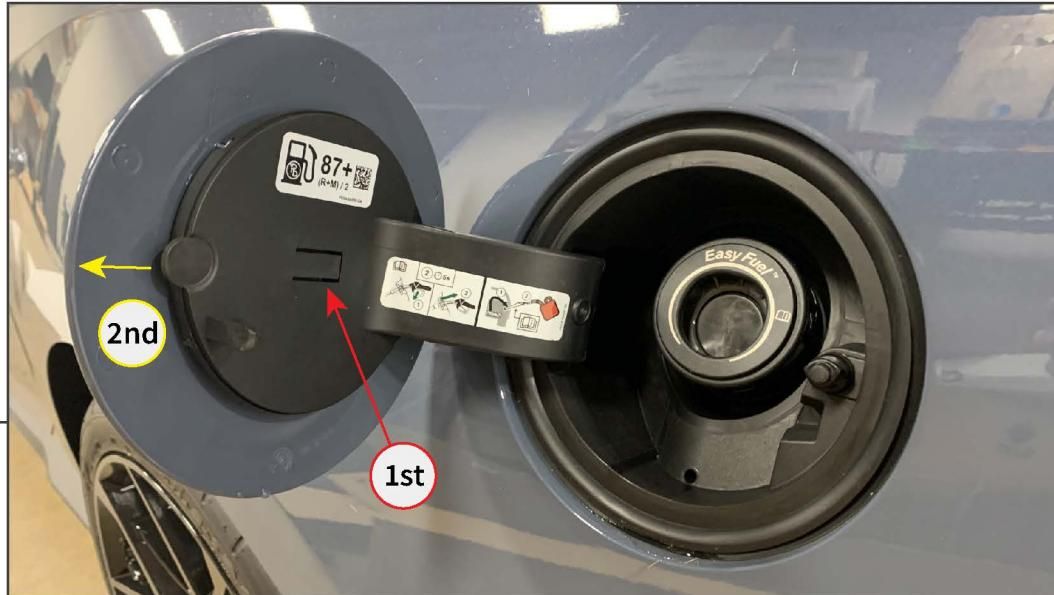
Open the vehicle fuel door. Locate the slot in the hinge panel. Using a flathead screwdriver/pry tool, gently pull back on the slot to disengage the fuel door lock tab. With the tab lifted, slide the fuel door off the hinge panel away from the vehicle.
