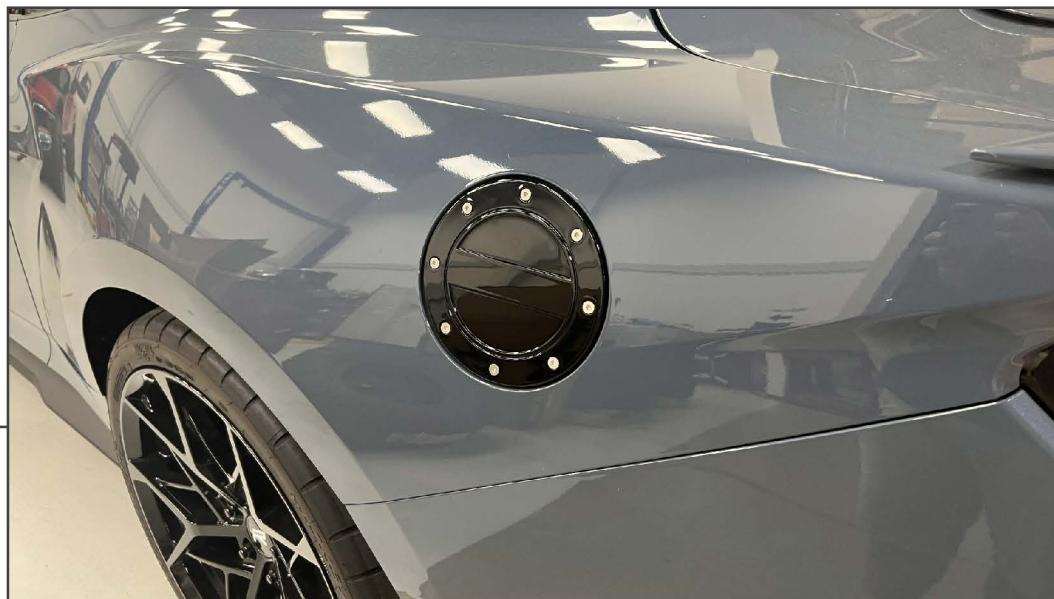
Carefully slide the new fuel door onto the hinge panel, ensuring all edges properly align into the guides. Fully slide the fuel door until fully seated. Slowly close the fuel door initially to ensure proper fitment.
