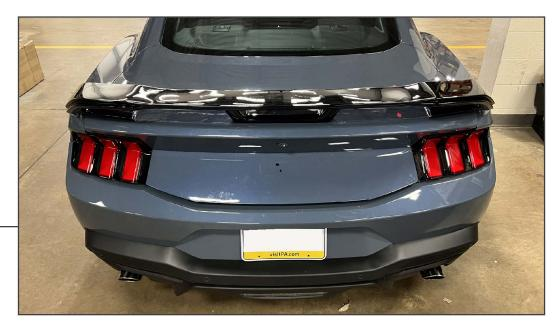
Re-install the vehicle backup camera, and the trunk panel inner core. Secure the inner core to the trunk panel using the original (6) T-15 Torx bolts. Plug in the backup sensor and secure the wiring harness in the original locations.
