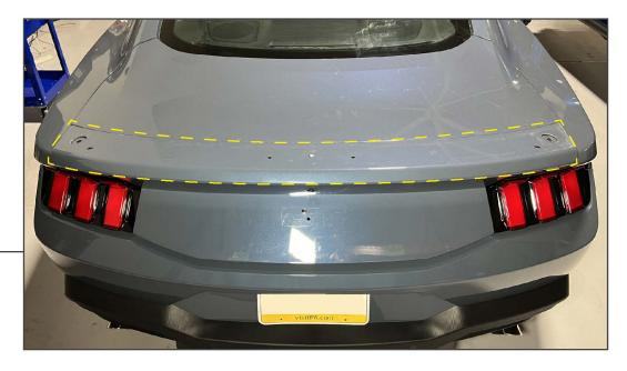
Clean the vehicle trunk lid using exterior detailer and a microfiber cloth.
