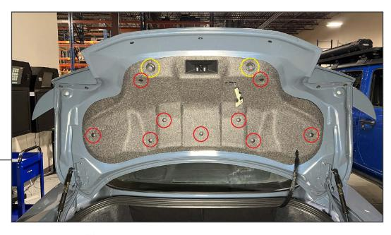
Open the vehicle trunk. Twist the (2) bump stops counter-clockwise to remove the bumpers from the trunk lid. Then, remove (9) plastic push clips from the trunk insulation.
