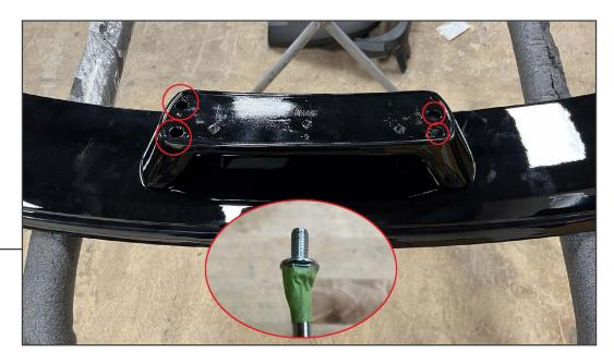
Secure the center support panel to the spoiler using (4) M6 flange bolts. (4) M6 lock washers, and (4) M6 flat washers. Tighten all hardware evenly until the center support is fully secure, do not over-tighten.
