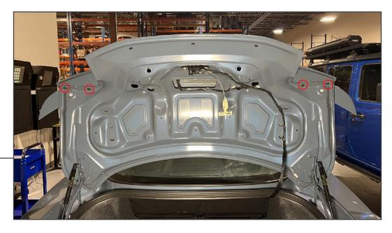
Remove (4) 7mm screws from the bottom of the trunk panel.
