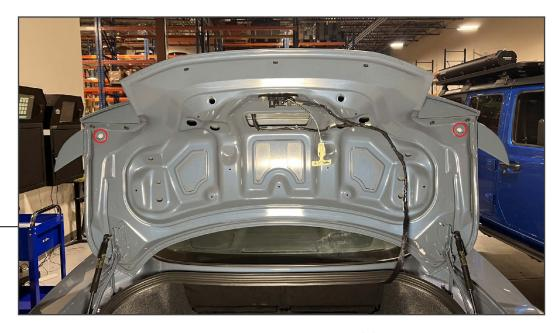
Remove (2) rubber grommets from each end of the trunk lid. Remove (2) 10mm bolts from the under-side of the vehicle spoiler.
