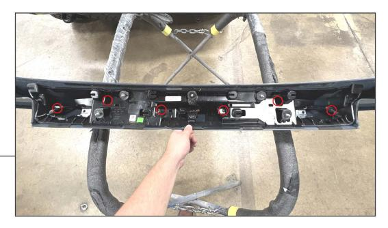
Remove (6) T-15 Torx bolts from the trunk panel inner core. With the bolts removed, use a plastic pry tool to dislodge the friction fit retainers around the trunk panel, and remove the panel inner core.
