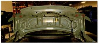
Remove (4) 7mm screws from the bottom of the trunk panel.
