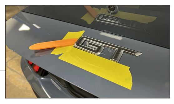
Place masking tape around the perimeter of the decklid emblem. Use a heat gun and heat the rear emblem to loosen the adhesive. Use a plastic pry tool to lift the emblem from the decklid.
