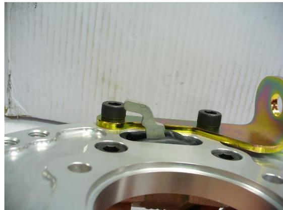
Figure 2b – Incorrect Cable Lever
