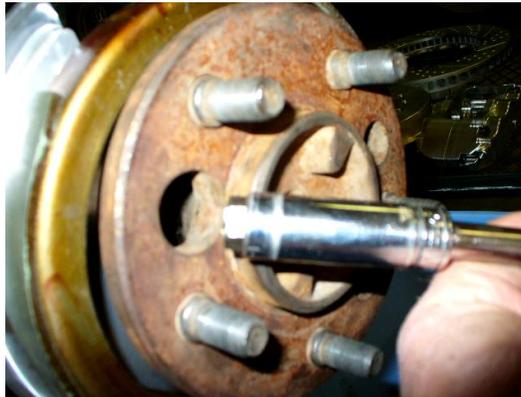
Figure 4 – Using the Access Hole
