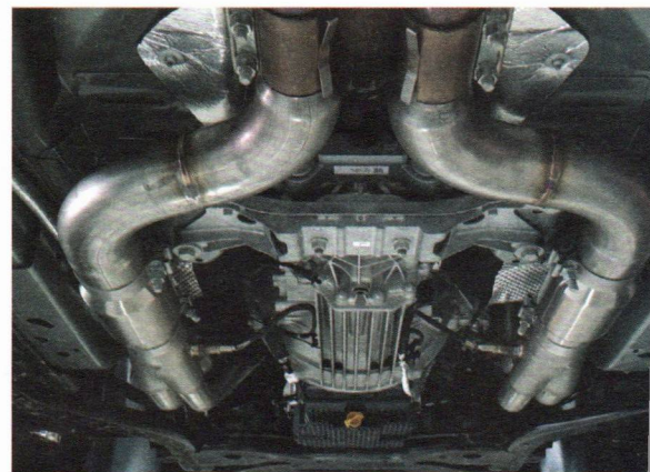
Detail 29: Catted headers installed to OEM catback connection
